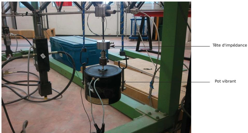
FIGURE 4.12 – Pot vibrant suspendu
