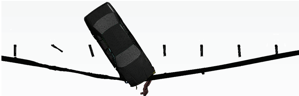
Figure 4- 3 Failure of vehicle redirection when H and E decrease greatly
