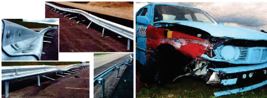
Figure 3- 6 Damage of the barrier and vehicle [60]
