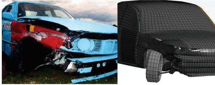
Figure 3- 16 Vehicle damages after crash test
