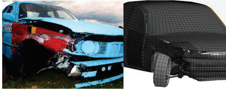
Figure 3- 16 Vehicle damages after crash test
