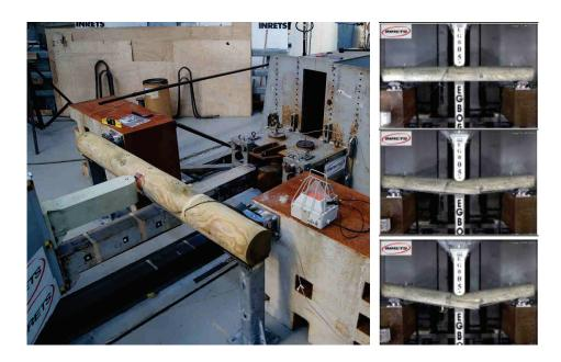
Figure 2-7 Bending test of steel reinforced wood beam [49]
