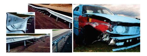
Figure 3- 6 Damage of the barrier and vehicle [60]
