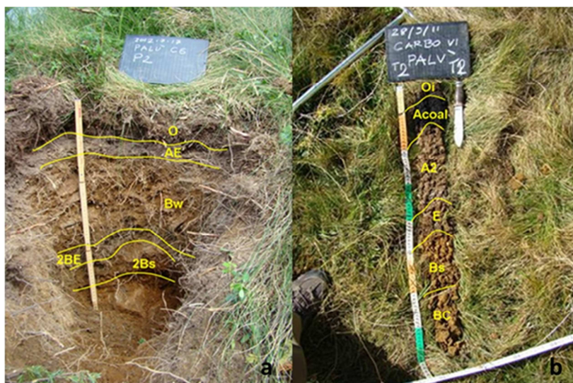
Figure III-1: Soil profile at the control site (Panel a) and the charcoal hearth (Panel b). The letters indicate different pedologic horizons. In the charcoal hearth the dark anthropogenic layer (Acoah; 0–10 cm) can be easily identified.
