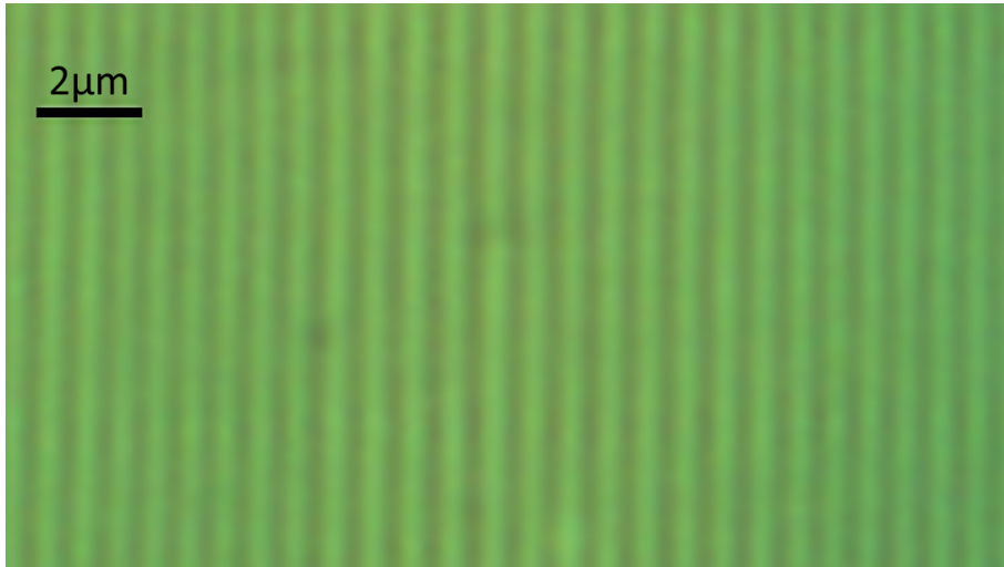
Figure 1.10: Photomicrograph of oily streaks, oriented at 45^\circ between crossed polarizers. The scale bar is oriented parallel to the easy axis.
