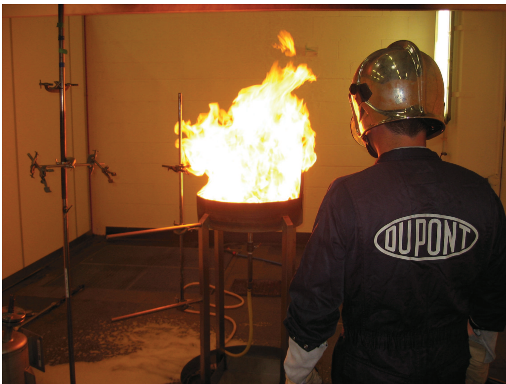
Figure 2.7: n-heptane fire for pilot firefighting water production (0.25 m 2 ).
