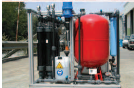
(c) Containerizable reverse osmosis plant. Source: http://www.polymem.fr
