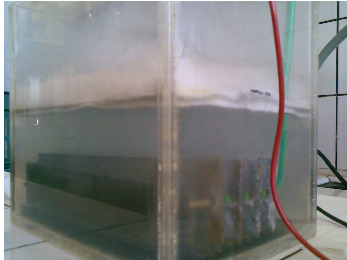
Figure 2.19: Floc layers during electrocoagulation of pilot firefighting water 2 at 2 A, after 30 min.
