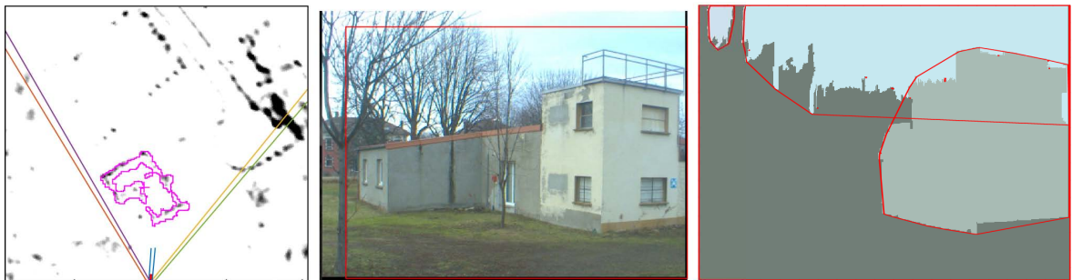
Figure 5.27: Example of the 3D reconstruction of the matched regions, with texture mapped into the 3D model.
