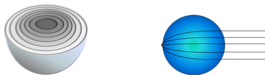
Figure 3.17: The shell layers are illustrated (a). An illustration of the wave reflection technique by the Luneburg lens with blue shading proportional to the refractive index (b).
