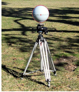
Figure 3.19: The detection of the center of the luneburg lens in the image. The circle corresponding to the spherical lens is first detected (red circle). Then the centroid of the detected circle is located (red cross).
