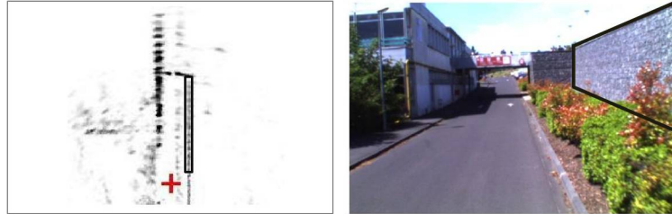
Figure 5.1: Example of regions matching between the camera image (right) and the radar panoramic (left): the black bounding box in the visual image should match the black bounding box in the radar panoramic. It can be seen visually that the regions in both images have common orientations of straight edges.
