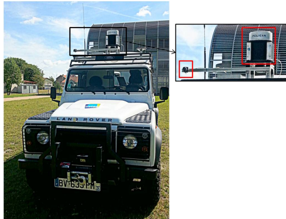
Figure 3.24: The radar and camera system is presented. (To the right) a zoom in on the sensors system is presented (the radar to the right and the camera to the left).
