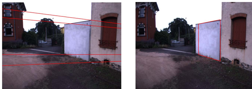
Figure 5.8: The epipolar lines in the left image corresponding to the corners pixels in the right image.
