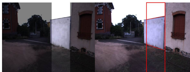
Figure 5.6: The red rectangle on the right image and its correlation (position of the corresponding rectangle) in the left image are shown.
