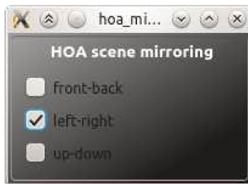
Figure D.9 hoa_mirroring compiled using faust2jaqt script. The checkboxes are used to select the mirror transformations among: left-right , front-back or up-down .
