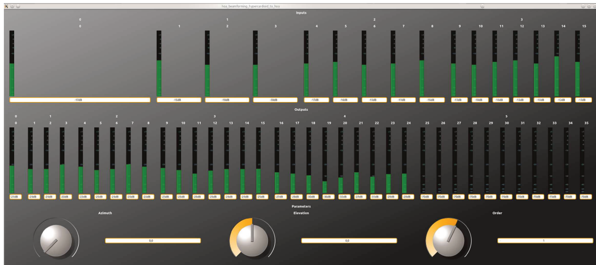
Figure D.15 hoa_beamforming_hypercardioid_to_hoa compiled using faust2jaqt script with M = 3 and M_1 = 2 . The VU-Meters at the top show the inputs signal levels in dBFS. The VU-Meters at the bottom show the outputs signal levels in dBFS. The knob Azimuth and Elevation are used to set the steering angles of the beampattern. Finally, the slider Order is used to set the hyper-cardioid order, from M_1 = 0 to M_1 = 2 in this case.
