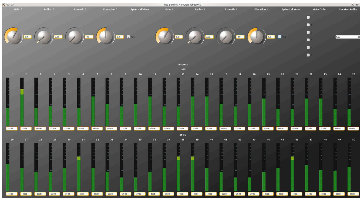
Figure D.7 hoa_panning_N_sources_lebedev50 compiled using faust2jaqt script with M = 5 and N = 2 . The slider Outputs Gain applies a global gain on all outputs (loudspeakers signals). The check-boxes Mute Order are used to mute some Ambisonic order in the computation of the driving signals. The sliders Gain Radius Azimuth Elevation control the position and gain of the sources. The check-box Spherical Wave is used to switch between the synthesis of a spherical wave or a plane wave. In the case of spherical wave synthesis, the input entry Speakers Radius sets the spherical loudspeakers system radius.
