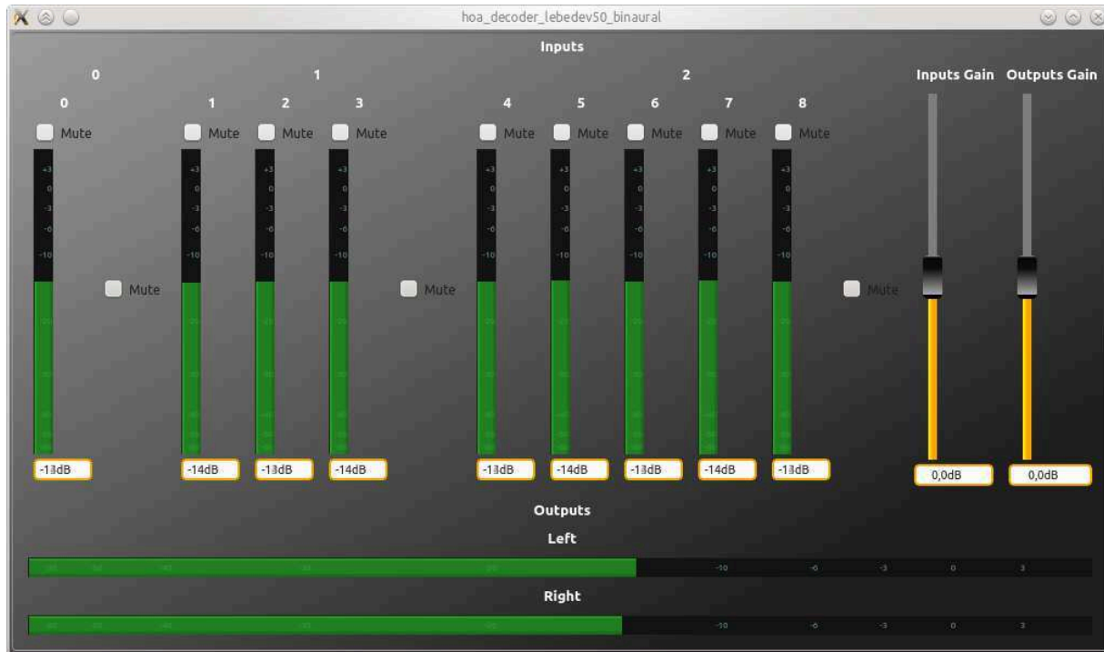
Figure D.6 hoa_decoder_lebedev50_binaural compiled using faust2jaqt script with M = 2 . The VU-Meters on top show the signal level of inputs Ambisonics components in dBFS. The check-boxes Mute are used to mute certain component or all components of an order. The slider Inputs Gain applies a global gain on all inputs. The slider Outputs Gain applies a global gain on all outputs. Finally, the horizontal VU-Meters at the bottom show the signal level in dBFS of Left and Right channels for headphone signal.
