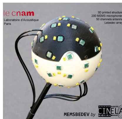
Figure 9: MemsBedeve microphone arrays with N = 50 MEMS microphones
