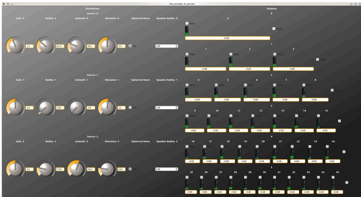
Figure D.2 hoa_encoder_N_sources plug-in compiled using faust2jaqt script with N = 2 and M = 5 . The Gain knob is used to adjust the input level of the input. Radius knob is used to set the source distance to origin in case of spherical wave encoding. Azimuth and Elevation knobs are used to set the source direction. The Spherical Wave check-box enables the encoding of spherical wave, using near-field filters. Speakers Radius sets the radius for the spherical array of loudspeakers at decoding stage in case of spherical wave encoding. Finally, the VU-Meters show the levels of 3D B -Format signals in dBFS up to order M . Each meter as a Mute check-box and each order as well.
