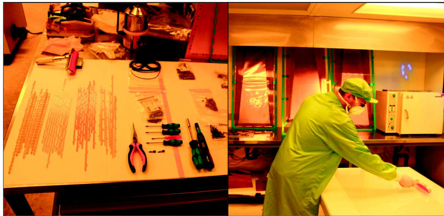
FIGURE B.1: Step 1: all the tools and components are prepared and carefully organized for the assembly (left). The working table, made of PolyMethyl MethAcrylate (PMMA), is cleaned with an adhesive roll (right).
