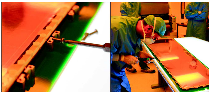
FIGURE B.12: Step 12: lateral screws are inserted in the brass pull-outs attached to the drift board until it reaches the embedded nuts (left). Then, torque control tools are used to stretch the foils, for a tension about 5 \text{ N/cm} .
