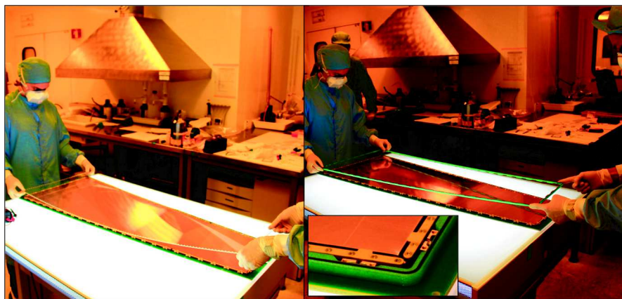
FIGURE B.14: Step 14: the PMMA protection cover is removed from the stack (left). Then, external frames equipped with the O-rings is placed around the GEM stack (right).
