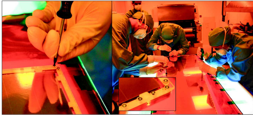
FIGURE B.9: Step 9: vertical screws are inserted into the frames in order to attach all the frame layers and GEM together.
