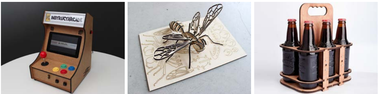
FIGURE 1.3 – An arcade ( thingiverse thing 1428410 ), a bee ( thingiverse thing 297758 ), and a pack of bottle laser cut ( thingiverse thing 16290 ). All those laser cut models require an assembly.
