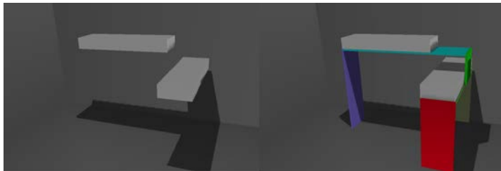
FIGURE 4.1 – Left : A Set of boxes in space placed by the user. Right : The synthesis is done by adding horizontal planks below each box and adding vertical planks to support the horizontal
