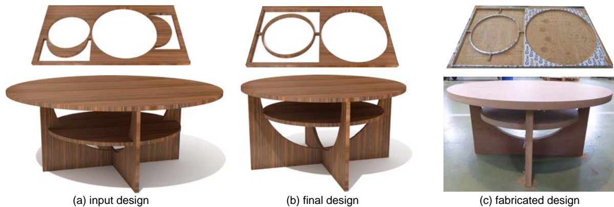
FIGURE 3.13 – We introduce waste-minimizing furniture design to dynamically analyze an input design (a) based on its 2D material usage (see inset) and design specifications to assist the user through (b) multiple design suggestions to reduce material wastage (see inset). The final user design can directly be exported for laser cutting and be assembled (c). In this case, wastage was reduced from 22% to 11%.
