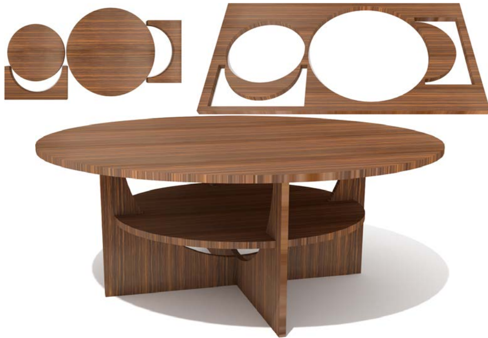
FIGURE 1.11 – Bottom :The model of a round table. Top Left : The cutting plan to cut the different part of this table. Top Right : The leftover of material after the cut.
