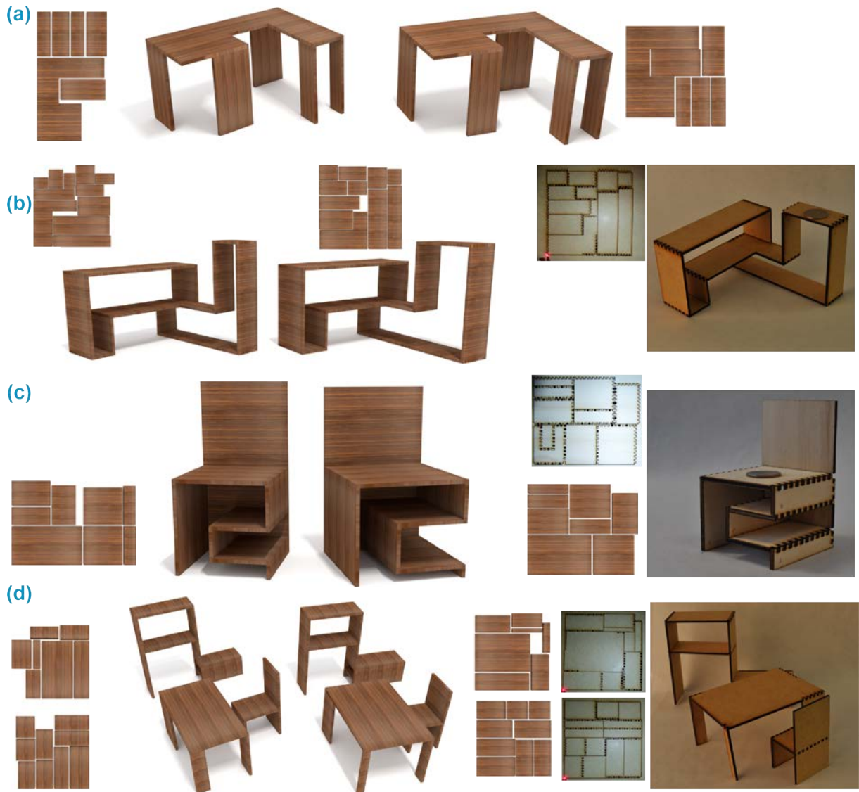
FIGURE 3.22 – Various material-driven design and fabrication examples. In each row, we show initial design (with material space layout inset), optimized design result (with material space layout inset), along with final cutout assembled model. Note that the design changes are often subtle, but still leads to significant improvement in material usage.
