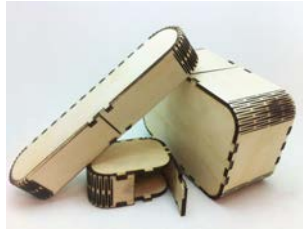
FIGURE 1.12 – Those boxes have been cut with a laser cutter. The pattern followed by the cutter allows some deformation that permit the user to close the boxes. ( Things 17240 from Thingiverse, user bdahlem )
