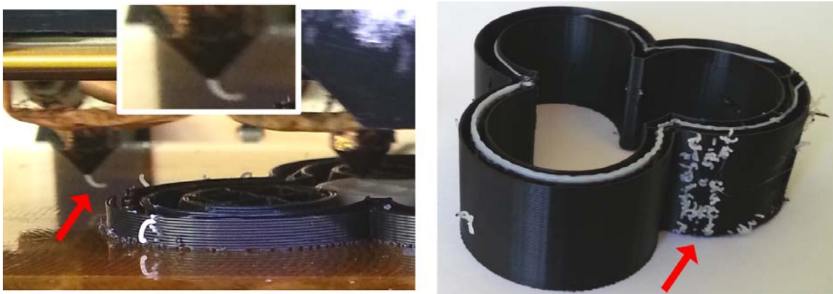
FIGURE 2.7 – Left : The 4–cones model printing. The red arrow shows how much ooze exits the left (white) nozzle while the right (black) nozzle prints. Right : The rampart captured a significant amount of stringing. Result shown Figure 2.6.
