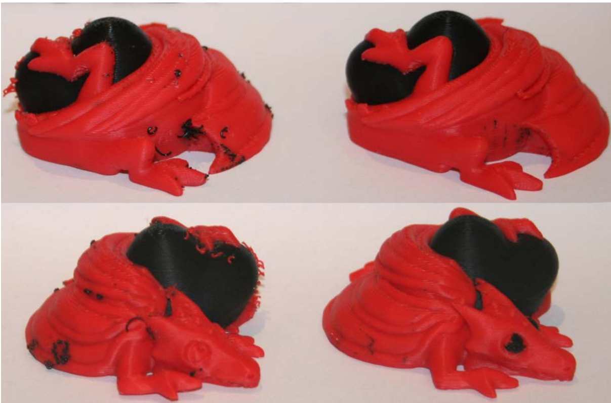
FIGURE 2.13 – Our result (right) has almost no defects compared to the same model printed with Skeinforge/ReplicatorG (left). Pictures focus on the worst regions of the surface. Both models use the optimized azimuth angle.
