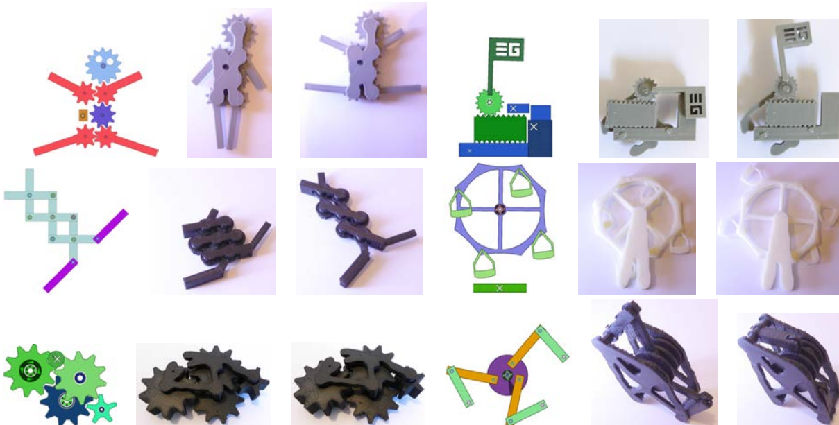
FIGURE 3.10 – A variety of results automatically generated from the input 2D design. All these results are 3D printed on filament printers.
