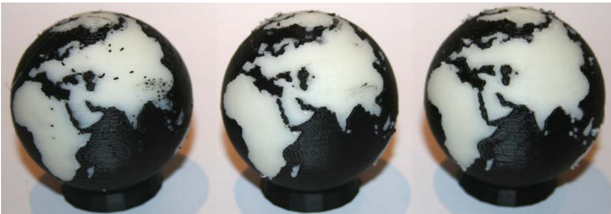
FIGURE 2.18 – From left to right : Two-color-world model, printed with ReplicatorG/Skeinforge, our technique without azimuth optimization and our complete technique.
