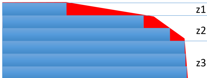
FIGURE 1.7 – The volumetric error (in red) depends of the gradient of the surface. The more horizontal it is, the bigger is the error. The zone shown in the figure presents the error in function of the gradient of the surface.
