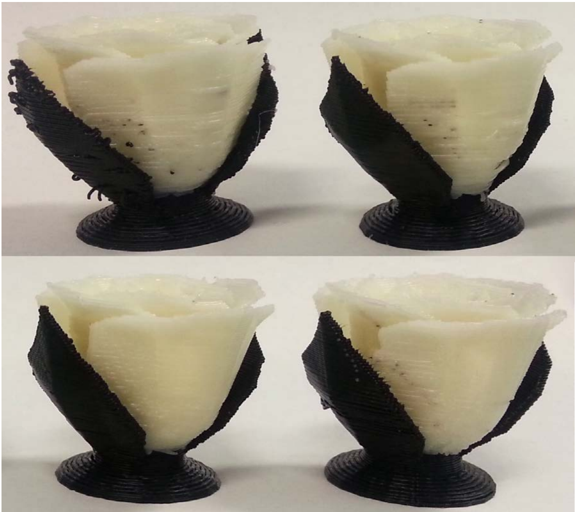
FIGURE 2.15 – Quality comparison. Top left : Print without our approach. Top right : Print with only the rampart (no navigation, no refill). Bottom left : Our final result. Bottom right : Print from Makerware 2.4. Rose by user Jillian (Thingiverse)
