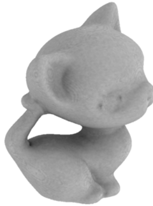
FIGURE 2.8 – The ambient occlusion computed on the kitten model. The algorithm uses darker area to hide defects where they are least visible. Thingiverse, thing 12694, user MBCook
