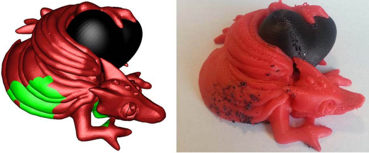
FIGURE 2.4 – The left extruder uses black and the right extruder red. While the red (right) extruder prints the body of the dragon, some black (left) plastic will interfere with the red region. This is accurately predicted by the intersection volume (green). The printed model exhibits severe color smears and strings throughout this volume. Additional defects are due to poor path planning.
