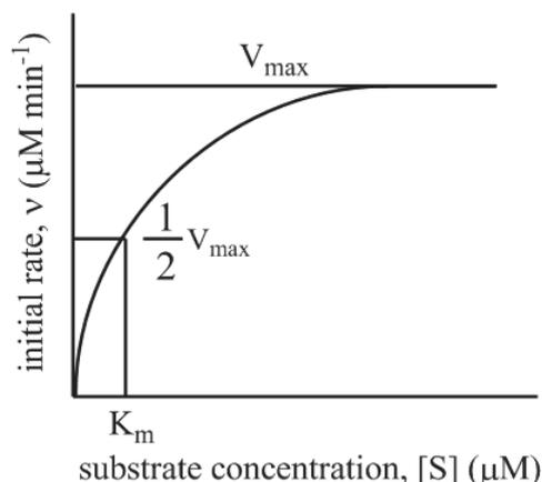
**Figure 9.** Plot of the initial reaction rate ( $v$ ) vs. substrate concentrations  $[S]$ .  $V_{\max}$  is represented as the maximal initial rate value from the enzymatic reaction, and  $K_m$  as the substrate concentration  $[S]$  where  $V_{\max}$  is the half
