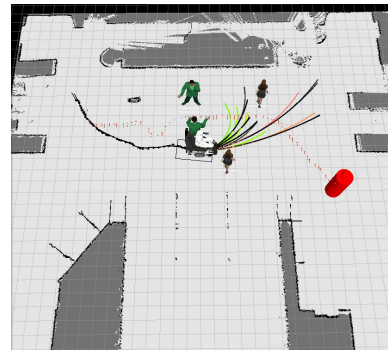
(d) when the obstacle is avoided the wheelchair keeps moving in the direction of the target.
