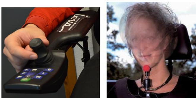
(a) Hand-operated joystick (b) A joystick operated with the chin.
