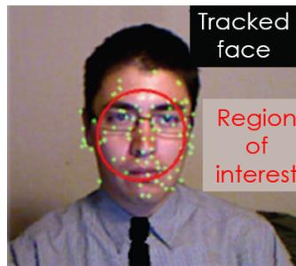
(a) The 2D RGB image is used to detect the face and fix a region of interest in the 3D point cloud.
