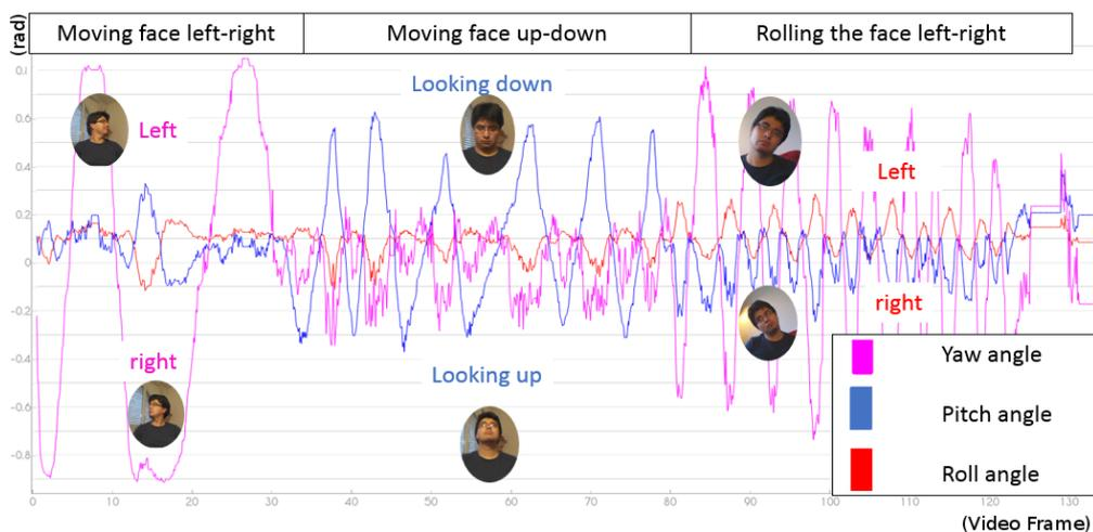
Figure 5.7: Face pose recognizer output angles. Yaw face's angle can be measured for movements in the range  $[-45^\circ, 45^\circ]$ ,  $pitch \in [-30^\circ, 30^\circ]$  and  $roll \in [-6^\circ, 6^\circ]$
