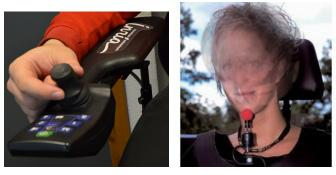
(a) Hand-operated joystick (b) A joystick operated with the chin.
