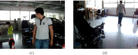
Figure 5.20: A scene of the robotic wheelchair following the user. This is an important characteristic that a robotic wheelchair should pursuit to ease the job not only for the user but also for the medical staff an his family.
