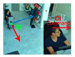
Figure 5.15: Using face pose to estimate the user's desired destination. (Video at http://goo.gl/VvtezQ).
