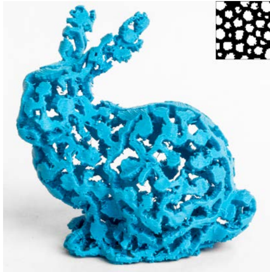
Figure 4.18 – This pattern is fully disconnected and therefore the appearance cannot be reconciled with the connectivity requirements of a sound structure. The produced object nevertheless prints correctly, and does capture some of the original features.
