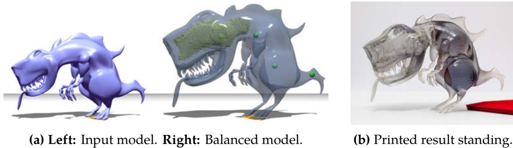
Figure 2.9 – Automatic shape balancing from [Prévost et al. 2013]. An unoptimized model is given as input to the system, which is allowed to slightly deform its surface, and carve its interior, to produce a balanced shape under the prescribed scenario (upright direction, contact points with the ground).
