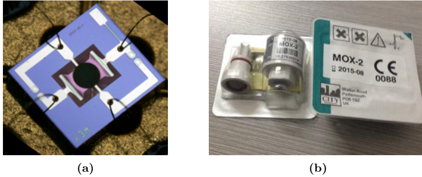
FIGURE 1.4 – Capteurs à oxyde métallique. (a) MSGS gas sensor, Microsens SA (b) CITY oxygen sensor, City Technology Ltd
