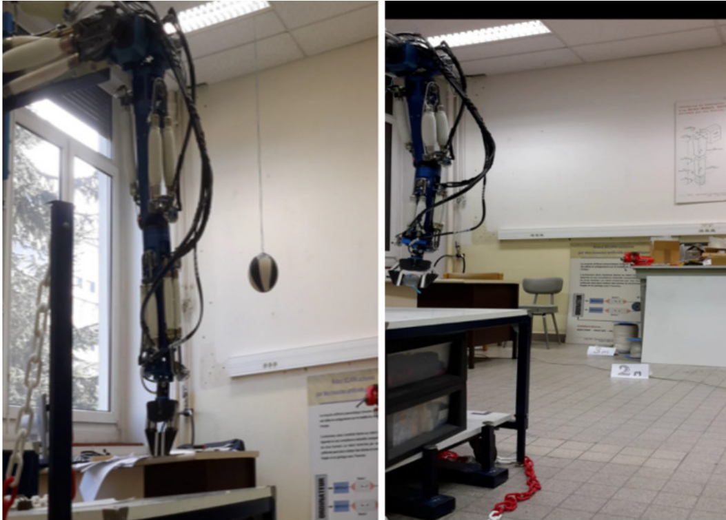
FIGURE 5.13 – Two experiments have been performed. Left picture is the set-up for the task of kicking the ball while the picture in right is the set-up for throwing the ball.
