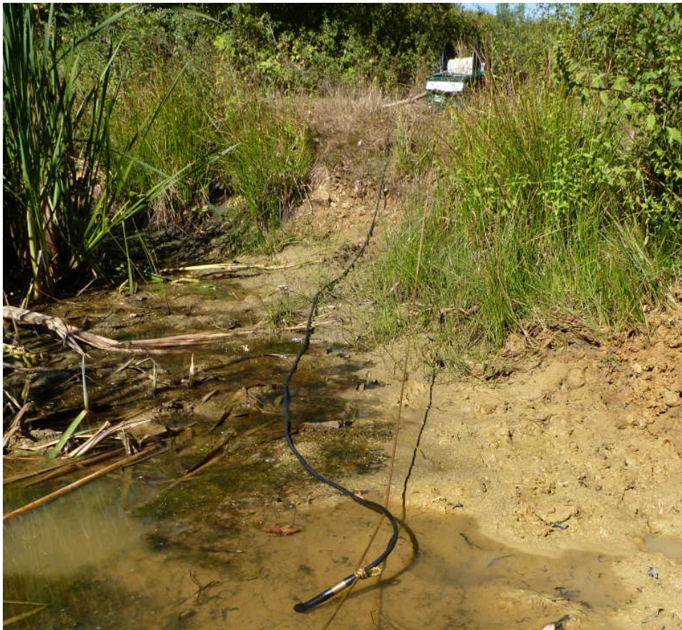
Hydrophone set up in pond 2, Vallée de Chevreuse (Yvelines, 78), June 2010 (Picture: Amandine Gasc)
