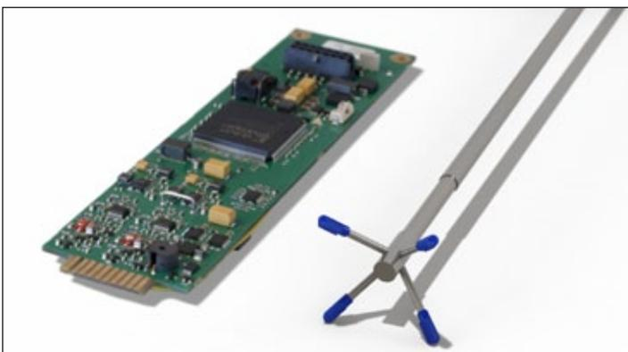
The Vectrino consists of two basic elements: the probe attached to a cylindrical housing and the processor inside the housing. From here the processed data is sent over a serial line or analog signals can be sent to an A/D converter.
