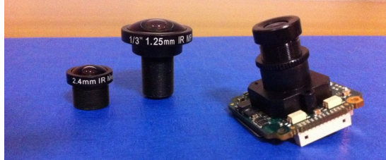
Figure 2.10: Matrix Vision mvBlueFOX-MLC usb camera.
