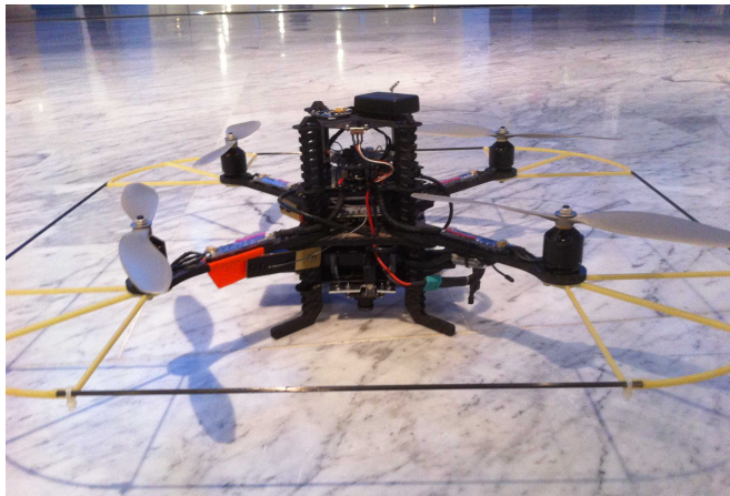
Figure 4.9: AscTec Pelican quadcopter [1] equipped with a monocular camera.
