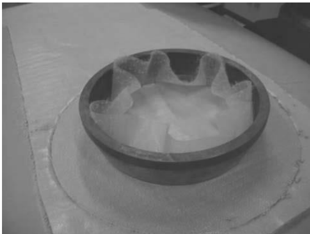
FIG. 4—Cutting the center of the mineral part of GCL 1 at a 0.2-m diameter.
