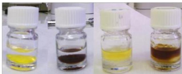
**Figure 4.1.** Yellow sample corresponds to QD530 and brown sample to QD705. Mutual colour change from (left) chloroform phase (bottom) to (right) aqueous phase (top).
