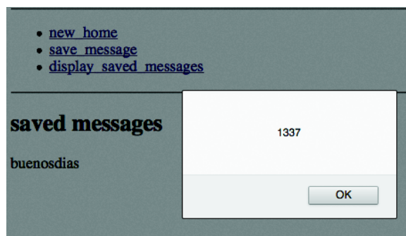
Figure 2.6: Successful exploitation of an XSS in the P0wnMe application
