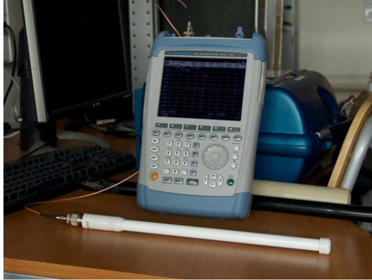
Figure 4.10: The Spectrum Analyzer FSH8 and the omnidirectional antenna ECO6-3500
