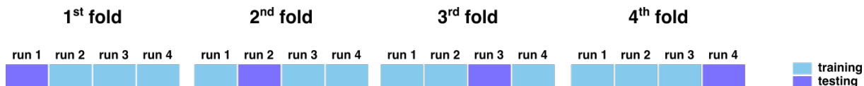
Fig. 6.1: 4-fold cross-validation process for assessing performance over the 4-class database for the discussed feature extraction methods in combination with the LDA and QDA algorithms, as well as for the distance-based approaches. Throughout each fold, the testing set (represented in dark blue) was constituted by all trials belonging to one of the runs (20 trials per class), and the training set (represented in light blue) was integrated by the remaining 3 runs (60 trials per class). After all folds, all possible choices are implemented and the performance scores for the 4 folds are averaged.
