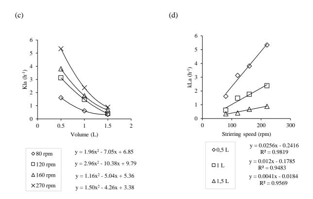
Figure 51: Relation between  $K_L a$  and (a) V for various  $\Omega$  for R- $\alpha$ . (b)  $\Omega$  for various V for R- $\alpha$ . (c) V for various  $\Omega$  for R- $\beta$ . (d)  $\Omega$  for various V for R- $\beta$ .
