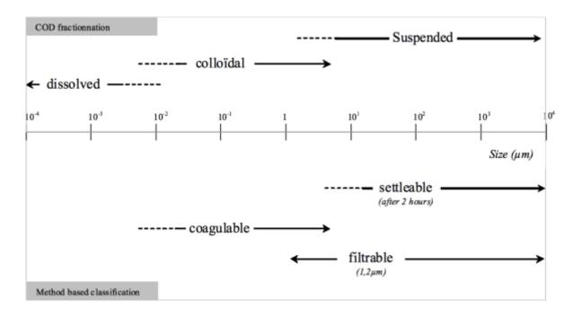
Figure 1: Wastewater fractionation with respect to particle size versus physical separation (Paul et al., 2012)
