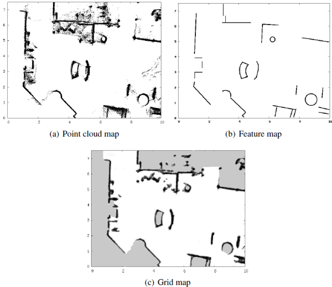
Figure 1.4: Examples of the three main approaches to perform map representation. The representation is based on lidar measurements.
