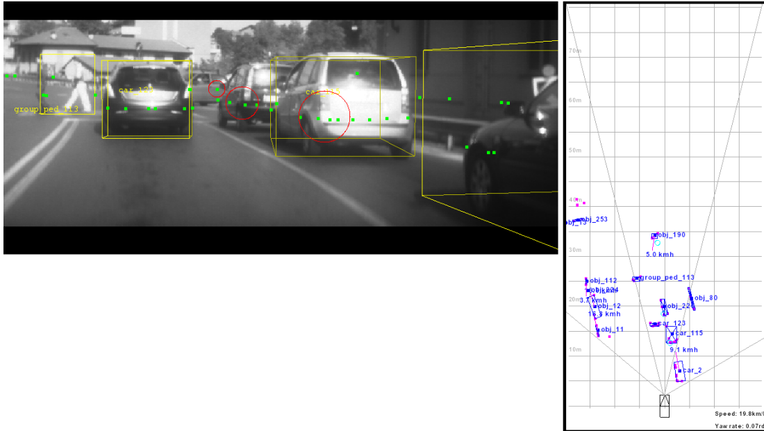
Figure 5.5: Results of the complete DATMO solution for urban areas. Several objects of interest are detected. Left side of the figure shows the camera image and the identified moving objects. Yellow boxes represent moving objects, green dots represent lidar hits and red circles represent radar detections. Right side of each figure shows the top view of the scene presented in the image. Objects classes are shown by tags close to each object.
