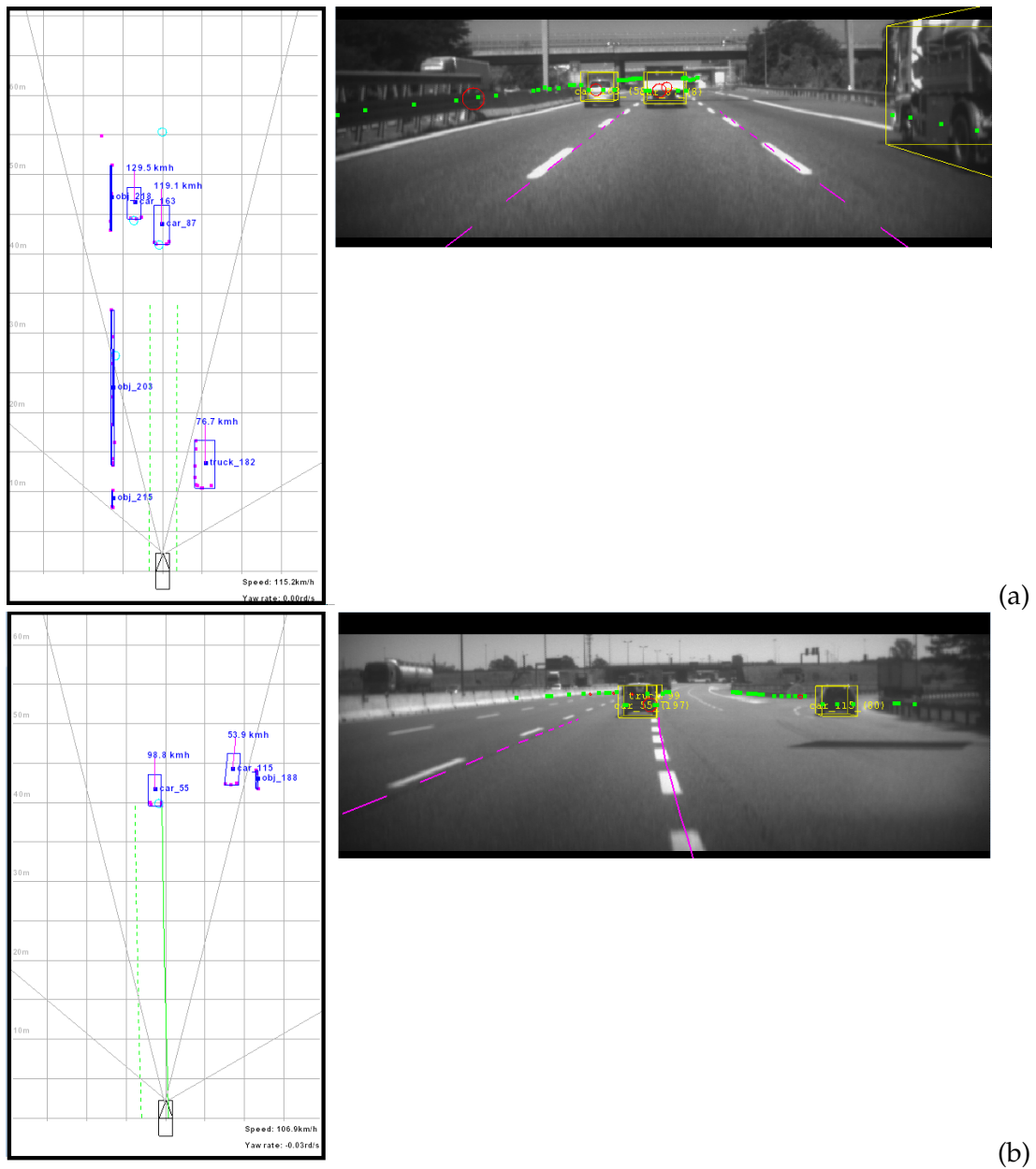
Figure 4.7: Results from the proposed fusion approach for moving object classification in (a,b) highway scenarios. The left side of each image represents the top view representation of the scene (static and moving objects) showed in the right-side image. Bounding shapes and class tags in the right side of each image represent classified moving objects.
