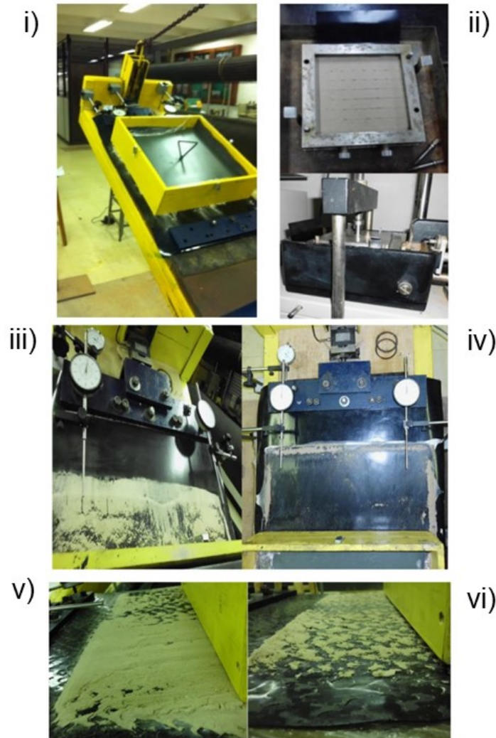
Figure 3.1.8. Soil-geosynthetic interface strength characterization on smooth and textured geomembrane interfaces: i) inclined plane and ii) conventional direct shear test; soil - smooth PVC geomembrane after inclined plane tests: (iii) degree of saturation of 5.5% and (iv) degree of saturation of 66%; soil - textured HDPE geomembrane after inclined plane tests: (v) degree of saturation of 5.5% and (vi) degree of saturation of 66% (modified from Monteiro et al., 2013).
