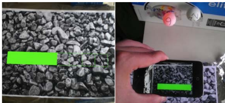
Figure 3.23: Prototype of an augmented light switch: (Left) the slider displayed on the handheld device's screen; (Right) the prototype system.
