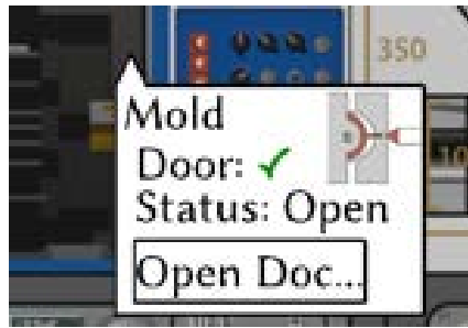
Figure 5.4: POI Frame component with Text and Image primitives and an 'Open Doc..' Button widget.
