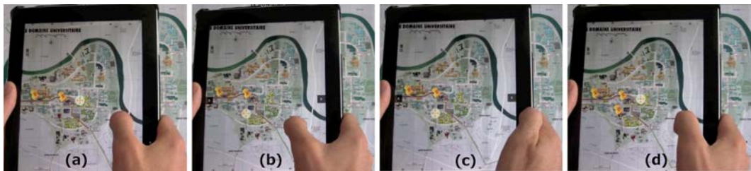
Figure 3.26: Relative Pointing : (a) we start with Crosshair ; (b-c) a finger stroke activates a precise relative pointing mode; (d) a tap on the screen performs selection and restores the Crosshair mode. The cursor was highlighted for better picture clarity.
