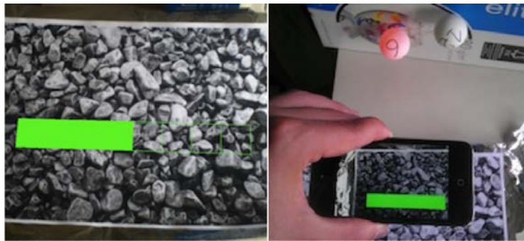
Figure 3.23: Prototype of an augmented light switch: (Left) the slider displayed on the handheld device's screen; (Right) the prototype system.
