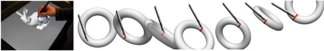
Figure 6.4: Direct drawing on 3D shapes with automated camera control: (Left) Drawing on a 3D shape on a tablet display with a stylus; and (Right) The camera viewpoint is adjusted to keep the stylus perpendicular to the shape, making it possible to draw across occluded and initially back-facing areas with a fairly constant precision.
