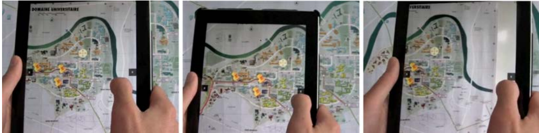
Figure 3.27: In the Relative Pointing mode, the cursor is stabilized on the remote physical object: moving the handheld device in space does not move the cursor on the physical object. The cursor was highlighted for better picture clarity.
