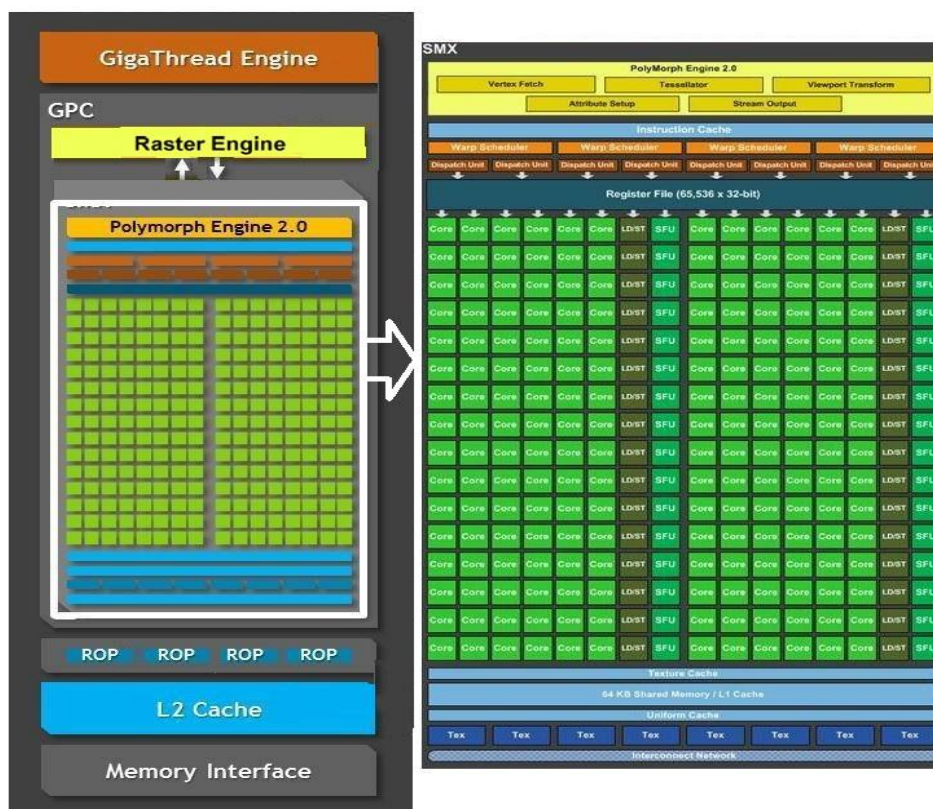
FIGURE 2.4 – Architecture Kepler du Tegra K1 [Nvidia, 2013].
