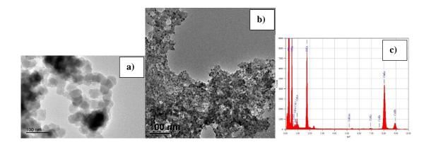
**Figure 5.5.** a) TEM image of silica NPs formed during the preparation of Co@SiO<sub>2</sub> NPs; b) TEM image of Co NPs encapsulated in a silica matrix; c) EDX spectrum showing a too high amount of silicon in the two samples
