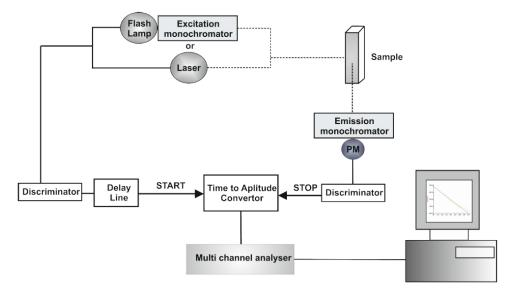
Figure 6.7. General setup for the measurements of lifetimes
