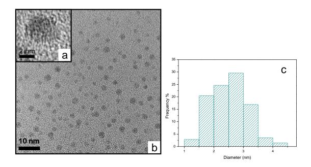
**Figure 2.4. a), b)** HR-TEM images of amine-terminated silicon nanoparticles obtained by microemulsion synthesis; in **a):** the crystal fringes of silicon are clearly visible; **c)** size distribution graph (average size  $2.5 \pm 0.6$  nm)
