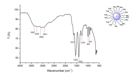
**Figure 2.9.** ATR-FTIR spectrum of amine-terminated Si NPs (microemulsion method); top right: model of a single nanoparticle. Peaks are assigned according to literature and IR tables<sup>[4, 14-16]</sup>
