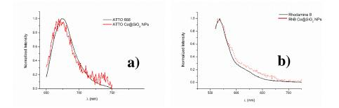
**Figure 5.16. a)** Emission spectra ( $\lambda_{exc} = 630 \text{ nm}$ ) in ethanol of free ATTO 655 (black line) and ATTO-Co NPs (red line); **b**) Emission spectra ( $\lambda_{exc} = 544 \text{ nm}$ ) in ethanol of free Rhodamine B (black line) and RhB-Co NPs (red line)
