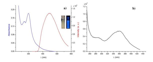
**Figure 2.6. a)** Absorption (blue) and emission (red) spectra of amine-terminated Si NPs (microemulsion method) in water ( $\lambda_{exc} = 300$  nm; filter 350 nm); inset: pictures of the solution under ambient illumination (left) and under UV irradiation (right); b) excitation spectrum in water ( $\lambda_{em} = 449$  nm).
