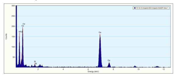
Figure 5.9. EDX spectrum of Co@SiO<sub>2</sub> NPs
