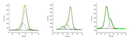
**Figure 2.18.** From left to right: Si2p, C1s and N1s high resolution regions of XPS spectrum of amine-terminated Si NPs made by hydrothermal synthesis. Experimental data in green, fitted spectrum in red, fit components in black.
