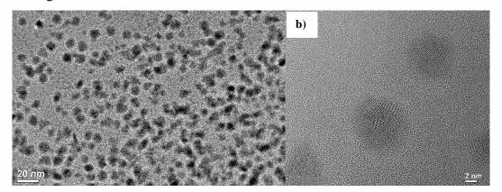
Figure 5.2. HR-TEM images of Co NPs; b) HR-TEM image at high magnification
