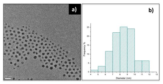
**Figure 5.6.** a) HR-TEM image of Co@SiO<sub>2</sub> NPs; b) size distribution graph (average size  $8.5 \pm 1.5$  nm) of Co@SiO<sub>2</sub> NPs
