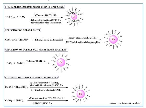
**Figure 1.18.** Four examples of bottom-up synthesis of ultrasmall cobalt nanoparticles  $(R = CH_3, C_2H_5, C_8H_{17}; trialkylphosphine = tributyl- or trioctylphosphine; DDAB = didodecyldimethyl ammonium bromide)$
