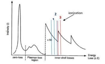
**Figure 6.3.** Illustration of the main features of an energy loss spectrum with indication of the energy windows used (three windows method) for obtaining elemental maps in EFTEM
