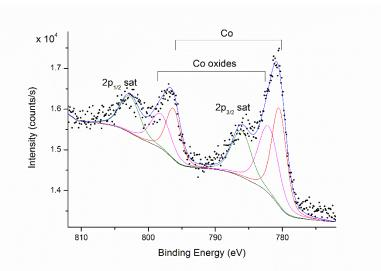
Figure 5.12. Co 2p region of the photoelectron spectrum of Co@SiO<sub>2</sub> NPs.
