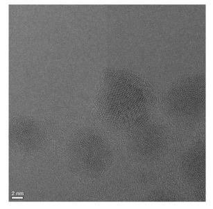
Figure 5.7. High magnification HR-TEM image of Co@SiO<sub>2</sub> NPs
