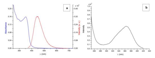
**Figure 2.15.** a) Absorption (blue) and emission (red) spectra of amine-terminated Si NPs (hydrothermal method) in water ( $\lambda_{exc} = 355$  nm); b) excitation spectrum in water ( $\lambda_{em} = 446$  nm).
