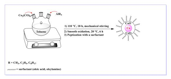
Figure 5.1. General scheme of the synthesis of cobalt nanoparticles
