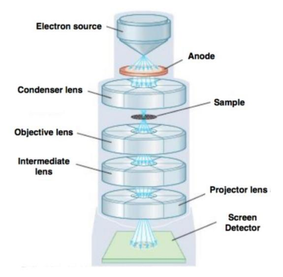
**Figure 6.1.** Schematic illustration of the basic components of an electron microscope A typical instrument is vertically arranged. The electron source is located at the top of the column and the electron beam reaches the sample after being focused on the sample plane through the condenser lens. Right after the sample, the object lens generates the intermediate image which is then magnified by the
