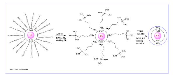
Figure 5.4. Synthetic route for the preparation of Co@SiO<sub>2</sub> NPs
