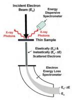
**Figure 6.2.** Scheme outlining the exploitation of inelastic scattering events for sample characterization
