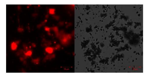
**Figure 5.17.** Confocal microscope images of ATTO-Co NPs ( $\lambda_{exc} = 630$  nm); on the right: bright field image showing NPs aggregates; on the left: detected emission ( $\lambda_{exc} = 630$  nm) of the ATTO 655 dye co-localized with NPs
