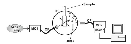
**Figure 6.5.** Schematic setup of an integrating sphere (MC = monochromator; OF = optical fiber, BT-CCD = back thinned CCD)
