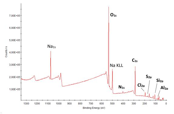
Figure 3.6. Survey XPS spectrum of s-Cy5-Si NPs.
