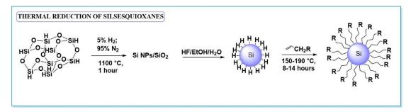
**Figure 1.10.** Thermal reduction of silsesquioxanes for the production of silicon nanoparticles (R = alkyl-, alkenyl-, amine-, epoxy-, alkoxy-, azide-groups, etc.)
