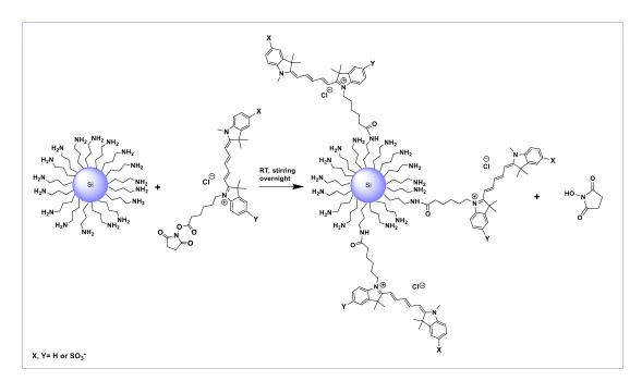
**Figure 3.3.** Synthetic route for the coupling of amine-terminated Si NPs with the dye cyanine 5 (X, Y = H) or its water-soluble analogue sulfo-cyanine 5 (X, Y =  $SO_3^{-1}$ )
