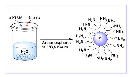
**Figure 2.11**. Schematic hydrothermal synthesis route for the preparation of amine terminated silicon nanoparticles. [APTMS = (3-aminopropyl) trimethoxysilane; citrate = Trisodium 2-hydroxypropane-1,2,3-tricarboxylate]
