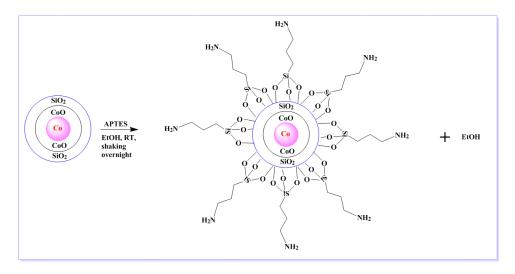
Figure 5.13. Amine functionalization of the Co@SiO<sub>2</sub> NPs
