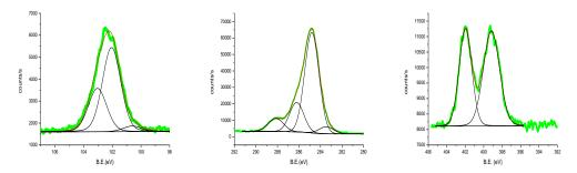
**Figure 2.10.** From left to right: Si2p, C1s and N1s high resolution regions of XPS spectrum of amine-terminated Si NPs made by the microemulsion technique. Experimental data are in green. The results of curve resolution are reported in red (resulting curve) and black (individual components).
