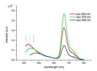
Figure 4.7. Emission spectra, in ethanol, of Cy5-CQDs at different excitation wavelengths
