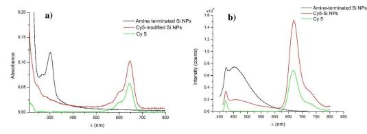
**Figure 3.5.** a) UV-vis and b) emission spectra ( $\lambda_{exc} = 375$  nm; filter 400 nm) in ethanol of a typical sample of amine-terminated Si NPs (black), Cy5-Si NPs (red) and of the free dye Cy5 (green)
