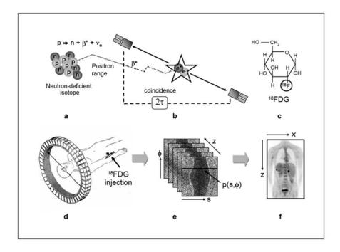
Figure 6.8. General setup of a PET scanner.
