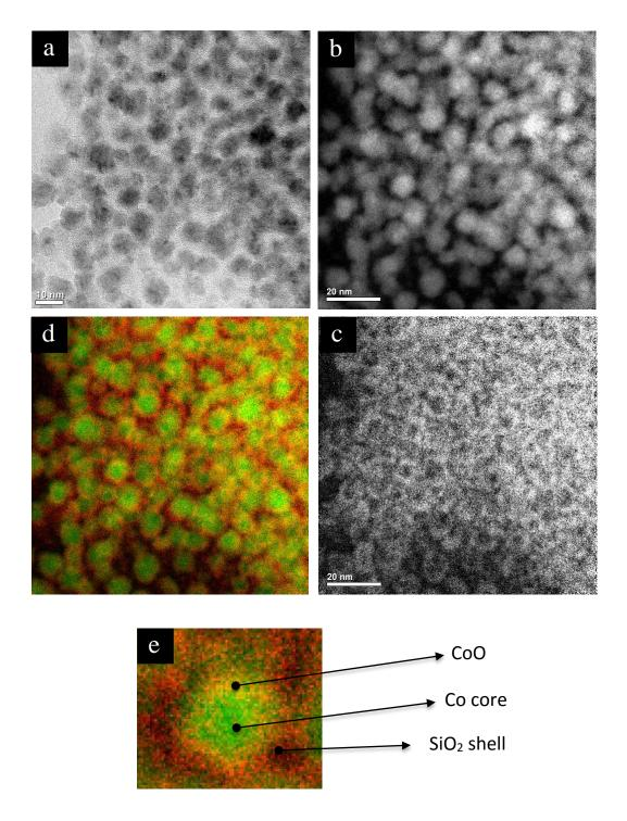
**Figure 5.10.** a) HR-TEM image of  $Co@SiO_2$  NPs; EFTEM maps of (b) cobalt and (c) oxygen; d) false colour overlay of (b) cobalt and (c) oxygen; images a), b), and c) are from the same region of interest with the same field-of-view; e) overlay image zoomed on a single particle.
