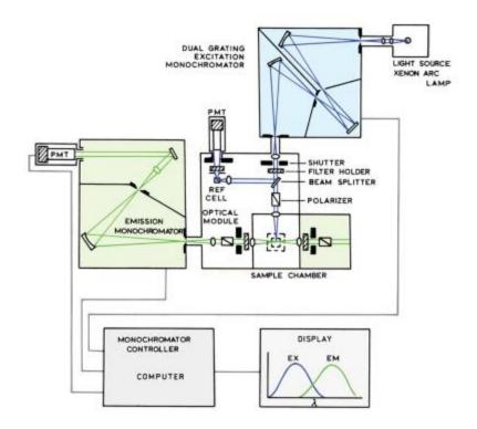
Figure 6.4. Schematic setup of a fluorimeter
