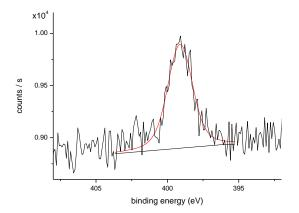
Figure 5.14. XPS core-level N1s spectrum of amine functionalized CO@SiO2 NPs
