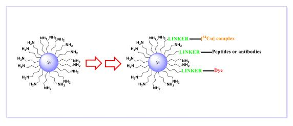
**Figure 3.2.** Schematic representation of some possible multi-functionalizations that can be carried on amine-terminated Si NPs
