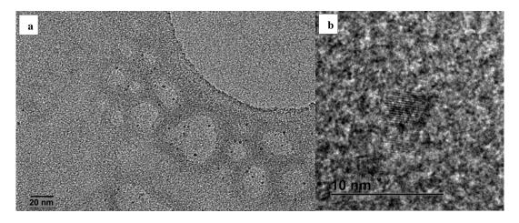
**Figure 2.12.** HR-TEM images of amine-terminated silicon nanoparticles obtained by hydrothermal synthesis; **15b:** an isolated NP presenting the crystal fringes of silicon.
