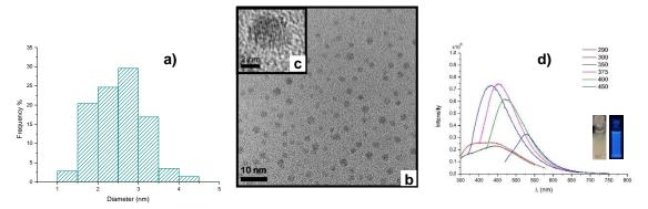
**Figure S1.** Main characteristics of amine-terminated Si NPs obtained by microemulsion technique: **a**) Size distribution graph (average size  $2.5 \pm 0.6$  nm); **b**), **c**) HR-TEM images, in **c**) the crystal fringes of silicon are clearly visible; **d**) Emission spectra at various excitation wavelengths in ethanol (the excitation wavelengths, in nm, are reported on the top right); inset: pictures of the solution under ambient illumination (left) and under UV irradiation (right)
