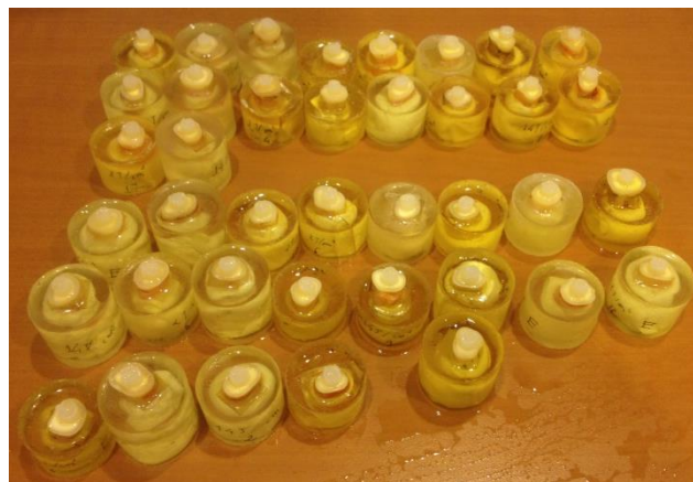
Figure 2.13: Photo of bonded specimens used for shear tests.
