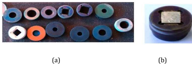
Figure 2-49: (a) sample holder with different shapes and sizes (b) Square sample holder with square shape sample.
