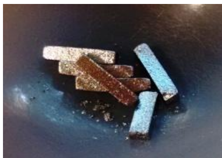
Figure 4-81: Picture representing the pellets of annealed sample \text{AgBi}_{0.7}\text{Sb}_{0.3}\text{Se}_2 .
