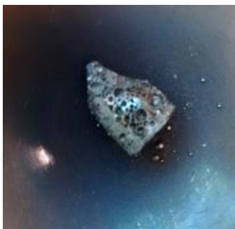
Figure 4-78: Picture of ingot; a solid chunk obtained after synthesis.
