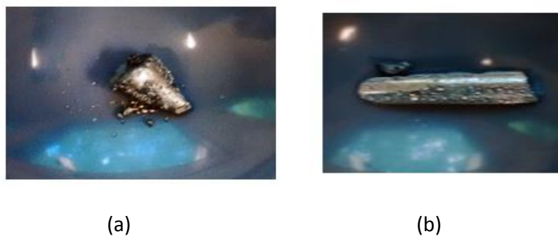
Figure 3-57: Ingot obtained after synthesis using (a) vertical furnace and b) horizontal cylindrical furnace.
