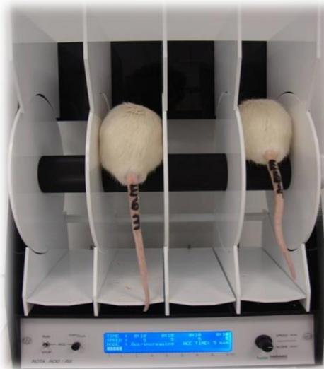
**Figure II-27.** The rotarod test device used in our experiment. It is based on a rotating rod with forced motor activity being applied by the rat. Supplier: Panlab/Harvard, Les Ulis, France.
