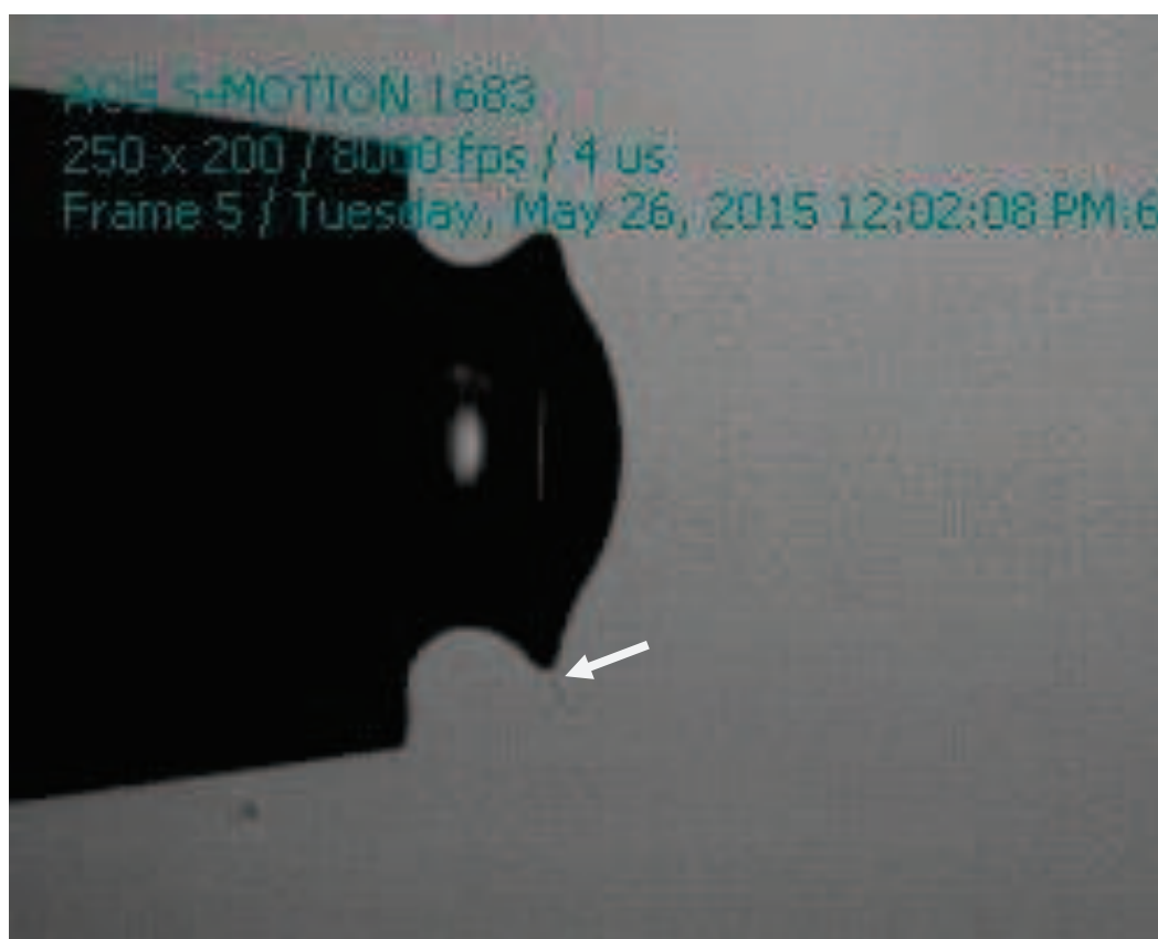
Fig 3.35. Jets off-axis produced from blunt-tip salted water meniscus for injection into Marcol 52 + 0.001 wt% Span 80 with MSP4, -5450V, h/R_{cap} = 0.75 (26/05/2015).
