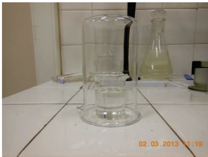
Fig 2.25. Marcol 52 pure in beaker is covered by another reversed beaker to avoid contamination by dusts.
