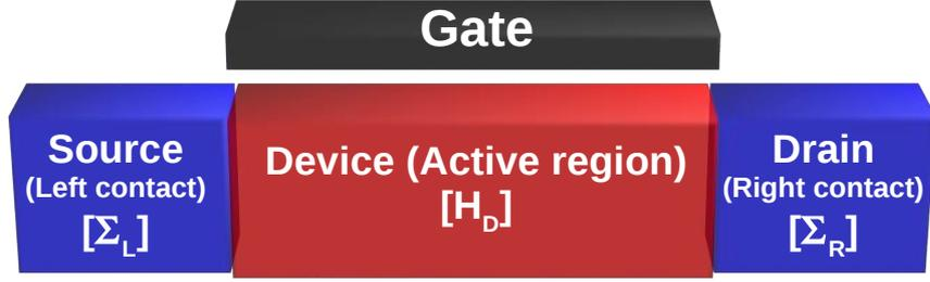
Figure 1.11: A general model of field effect transistor with a device channel connected to the source and drain contacts. The electrical current is modulated by a third electrode, the gate. The coupling to contacts is described by  $\Sigma_{L,R}$  self energy.
