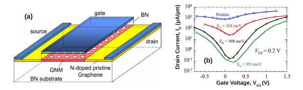
Figure 3.5: Schematic view of the GNM transistor is considered in figure (a). Transfer characteristics is displayed in figure (b) [92].
