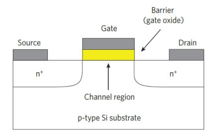
Figure 3.2: Schematic of conventional field-effect transistor [107].
