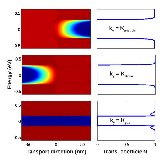
Figure 2.25: Local density of states (left panels) and corresponding transmission coefficient (right panels) for three different wave-vectors  $k_y$  obtained in an unstrained/strained graphene junction of  $\sigma = 5\%$  and  $\theta \equiv \phi = 0$ .
