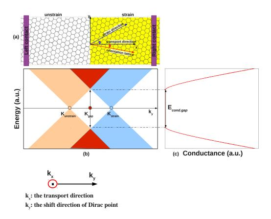
Figure 2.23: (a) unstrained/strained graphene junctions. (b) bandedges illustrating the strain-induced shift of Dirac points along the  $k_y$ -direction that leads to the opening of a conduction gap (c).
