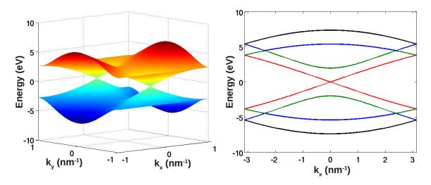
Figure 2.3: Electronic bandstructure in graphene lattice. Left panel: the full energy spectrum in 3 dimensions. Right panel: the energy bands along  $k_x$  direction.
