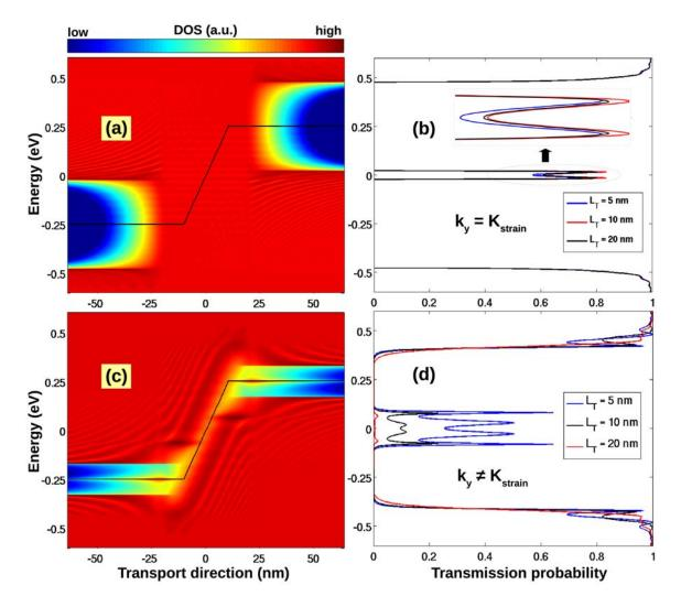
Figure 3.31: Maps of local density of states (left) and corresponding transmission probability (right) obtained for two different wavevectors  $k_y$ . In the right side, devices with different lengths  $L_T$  are considered. The inset in (b) shows a zoomed image of the transmission probability around the zero energy point. Other device parameters:  $L_S = 40$  nm,  $\sigma = 3$  % and  $U_0 = 0.5$  eV.
