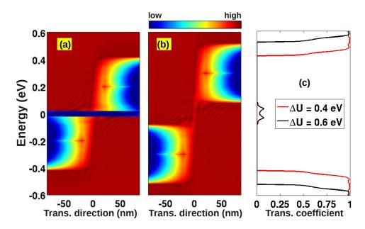
Figure 3.20: Local density of states in the devices of different  $\Delta U$ : 0.4 (a) and 0.6 eV (b) (the blue color regions correspond to energy-gaps, i.e., low density of states). The transmission coefficient in these cases is shown in (c).  $k_y = (K_y^{unstrain} + K_y^{strain})/2$  and  $\sigma = 5\%$  are considered here.
