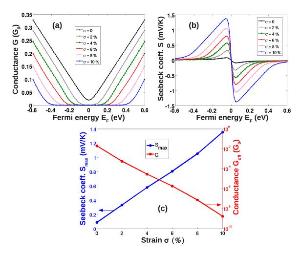
Figure 3.14: (a) Conductance and (b) Seebeck coefficient as a function of Fermi energy  $E_F$  for different strain amplitudes in the device with uniform doping. (c) Maximum value of Seebeck coefficient  $(S_{max})$  and conductance  $(G_{off})$  in OFF state (i.e., at  $E_F = 0$ ) as a function of strain amplitude.
