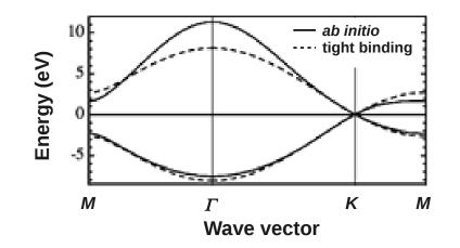
Figure 1.10: Ab initio and nearest-neighbor tight-binding dispersions of graphene. The converged ab initio calculation of the graphene  $\pi$  and  $\pi^*$  electronic bands is shown by the full lines. The dashed lines represent the tight-binding dispersion of Eq. 1.46 with s = 0 and t = 2.7 eV [57].
