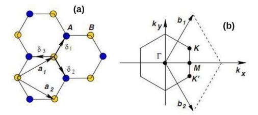
Figure 1.8: Graphene lattice and its Brillouin zone. (a) lattice structure of graphene, made out of two interpenetrating triangular lattices  $(\vec{a_1} \text{ and } \vec{a_2} \text{ are the lattice unit}$ vectors). (b) corresponding Brillouin zone with two reciprocal lattices  $\vec{b_1}$  and  $\vec{b_2}$ . The Dirac cones are located at the K and K' points [3].
