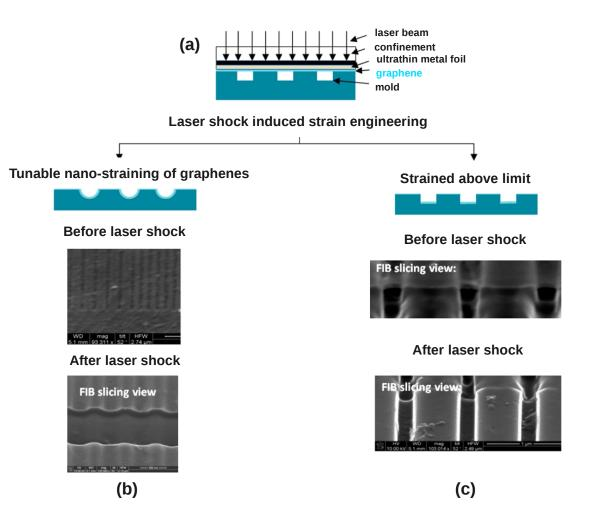
Figure 1.7: Illustration of the laser shock induced straining of graphene [44]. (a) setup of of the laser-induced strain engineering, (b) tunable 3D nanostraining of the graphene film when the strain limit is not exceeded. (c) graphene straining above the strain limit.
