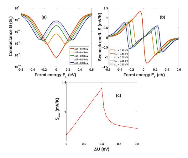
Figure 3.19: (a) conductance and (b) Seebeck coefficient as a function of Fermi energy  $E_F$  with high values of  $\Delta U$ . The relationship between  $S_{max}$  and  $\Delta U$  is shown in (c).  $\sigma = 5\%$  is considered here.
