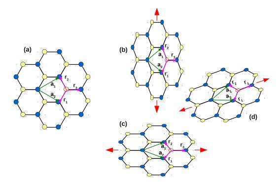
Figure 2.15: Graphene (a) and strain graphene (b, c, d). The strain is applied along a zigzag axis in (b), a armchair axis in (c) and any axis in (d).
