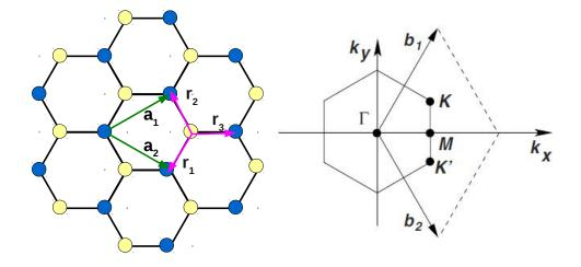
Figure 2.1: Honeycomb lattice of graphene and its Brillouin zone. Left panel: lattice structure made out of two triangular lattices ( $\vec{a}_1$  and  $\vec{a}_2$  are the unit vectors, and  $\vec{r}_1, \vec{r}_2, \vec{r}_3$  are the nearest-neighbor vectors). Right panel: Brillouin zone in reciprocal space. The Dirac cones are located at the K and K' points.
