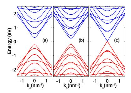
Figure 2.5: Electronic structure of armchair graphene nanoribbon is shown in three cases. (a) and (b) are semiconducting corresponding with n = 3p and n = 3p + 1, respectively. (c) with n = 3p + 2 is metallic (p: an integer number).
