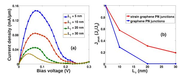
Figure 3.30: I-V characteristics of the device with different lengths  $L_T$  while  $L_S = 40$  nm is fixed in (a). The evolution of peak current  $J_{peak}$  when increasing  $L_T$ , compared to that in the case of normal semiconducting (gapped) graphene channel in (b), where  $J_0$  is the current obtained for  $L_T = 5$  nm. Other parameters:  $\sigma = 3\%$  and  $U_0 = 0.5$  eV.
