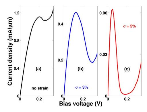
Figure 3.23: I - V characteristics of a single potential barrier structure for different strain amplitudes. Other parameters of the structure are:  $L_S = L_B = 40$  nm,  $U_0 = 0.45$  eV, and  $E_F = 0.25$  eV.
