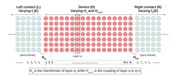
Figure 1.12: Layered description of a device.
