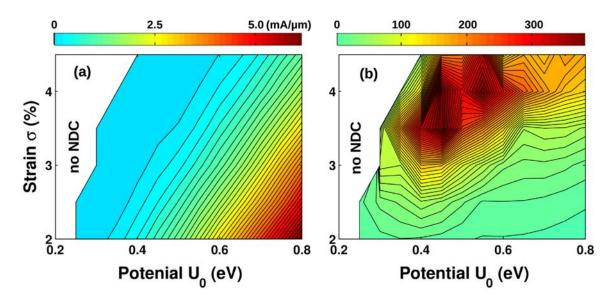
Figure 3.29:  $(\sigma - U_0)$  maps of peak current (a) and PVR (b) in the p-n junction with  $L_S = 40$  nm and  $L_T = 10$  nm.
