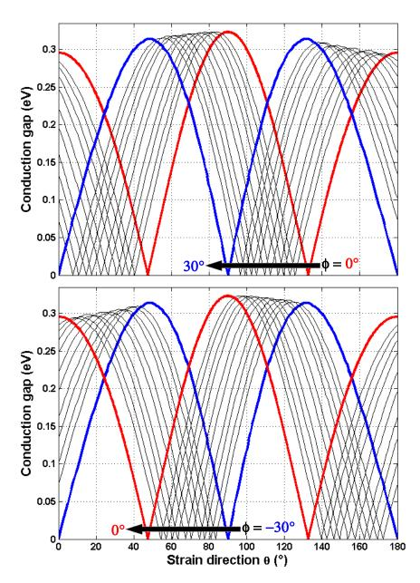
Figure 2.33: Dependence of conduction gap on the directions  $(\theta, \phi)$  for  $\sigma = 4\%$ .
