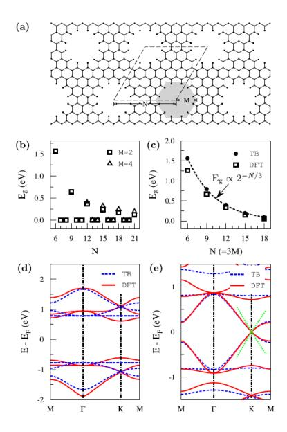
Figure 2.12: (a) Schematic of a triangular graphene antidot lattice. The unit cell indicated by dashed lines can be characterized by (N, M), where N is the periodicity and M is the side length of the hexagonal hole. (b) The variation of bandgaps as a function of N with M = 2 and M = 4. (c) The variation of bandgaps as a function N with M = N/3. (d) The band structure of a (6, 2) antidot lattice. (e) The band structure of a (7, 2) antidot lattice. From A. Zhang *et al.* [69]
