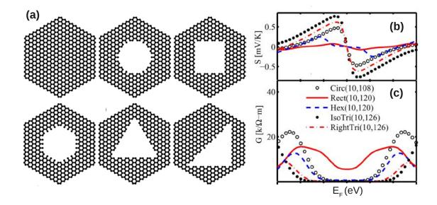
Figure 3.12: Geometrical structures of different graphene antidot lattices (GALs) in (a) with Circ(10, 108), Rect(10, 120), Hex(10, 120), IsoTri(10, 126), and RightTri(10, 126), respectively. Seebeck coefficient and electrical conductance are displayed in figure (b) and (c). From H. Karamitaheri *et al* [133].
