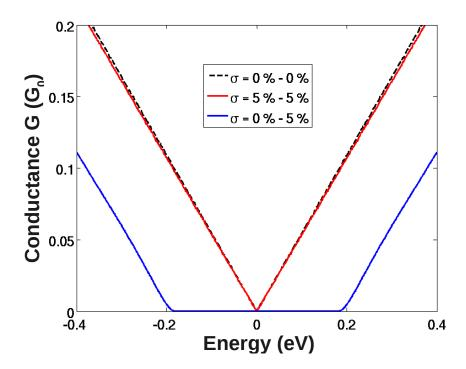
Figure 2.24: Conductance  $(G_0 = e^2 W/hL_y)$  as a function of energy in strained graphene heterostructures. The comparison of the conductance in unstrained, uniformly strained and strained heterostructures is shown. The transport along the armchair direction ( $\phi = 0$ ) with a strain applied along the Ox axis ( $\theta = 0$ ) are considered here.
