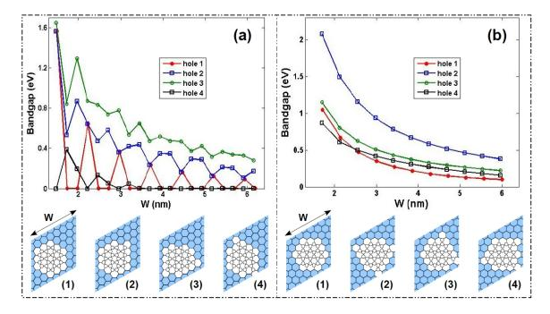
Figure 2.13: Energy gap of GNM lattices as a function of the super-cell lattice constant for different hole shapes. (a) is for zigzag holes while (b) is for armchair holes. The super-cells of considered GNM lattices, where white circles indicate the removed carbon atoms, are presented in the bottom of the two sub-figures. From Nguyen *et al.* [98]
