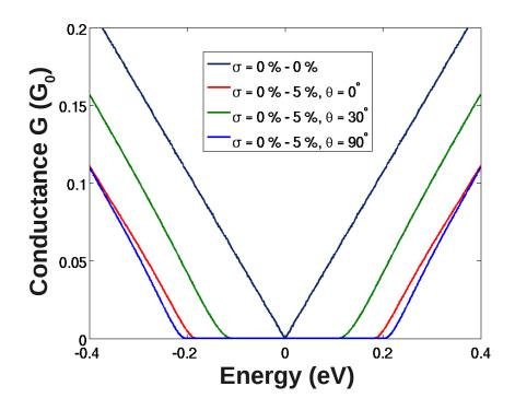
Figure 2.26: Conductance  $(G_0 = e^2 W/hL_y)$  as a function of energy in graphenestrained junctions for = 5% with different strain directions. The transport along the armchair direction  $(\phi = 0)$  is considered. The data obtained in a uniformly strained graphene are displayed for the comparison.
