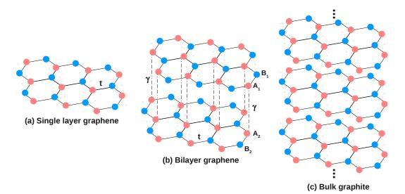
Figure 2.8: Lattice structure of single layer (a), bilayer graphene (b) and bulk graphite (c). t and  $\gamma$  are hopping parameters. The A and B sublattices are indicated with index 1,2 as shown in figure.
