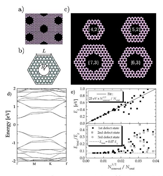
Figure 2.11: Illustration of the triangular antidot lattice (a) with a unit cell characterized by side length L and hole radius R (b). In (c), several examples with corresponding (L, R) parameters are shown. In (d), energy band structure for a (7,3) antidot lattice. (e) compilation of energy gaps, displayed versus  $\sqrt{N_{removed}}/N_{total}$ , very simple scaling is observed. From T. G. Pedersen *et al.* [93]
