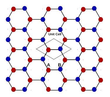
Figure 1.9: Graphene lattice is composed of two triangular sub-lattices A and B. Unit cell is shown in figure with two atoms. It is noted that the lattice constant is a $(a = 1.42A^{\circ})$ .
