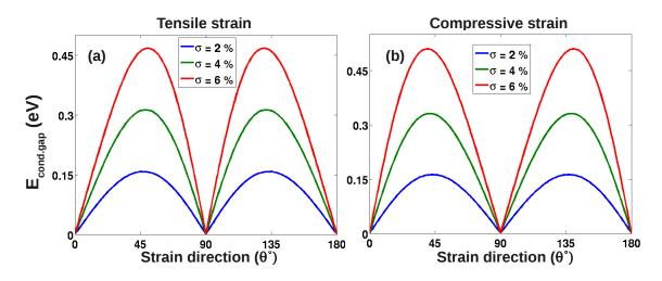
Figure 2.28: Maps of conduction gap in unstrained/strained graphene junctions: tensile (a) and compressive cases (b). The transport is along the zigzag directions,  $\phi = 30^{\circ}$ . The strain of 2%, 4%, 6% is considered.
