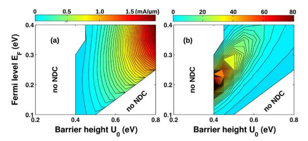
Figure 3.26:  $(E_F-U_0)$  maps of peak current (a) and PVR (b) in the single potential barrier structure with  $L_S = L_B = 40$  nm and  $\sigma = 5\%$ . Other parameters:  $E_F = 0.25$  eV,  $U_0 = 0.45$  eV, and  $\sigma = 5\%$ .
