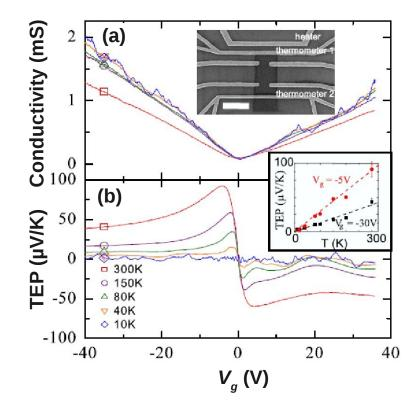
Figure 3.9: (a) Electrical conductivity and (b) themoelectric power (TEP) of a graphene sample as a function of Vg (for different temperatures) for single graphene. From Y. M. Zuev *et al* [62].
