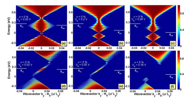
Figure 3.24:  $(E-k_y)$  maps of transmission probability in two cases of unstrained (top) and strained (bottom) devices with different applied bias.  $K_0$  denotes the position of Dirac point of unstrained graphene and  $U_0 = 0.45$  eV is considered here.
