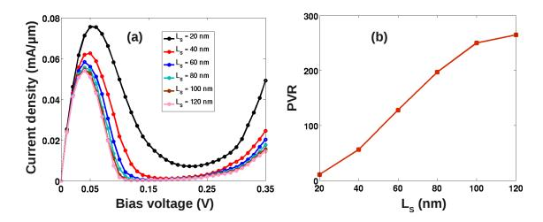
Figure 3.27: I - V characteristics computed for different lengths of strained region  $L_S$  (a). The PVR as a function of  $L_S$  is shown in (b). Other parameters:  $E_F = 0.25$  eV,  $U_0 = 0.45$  eV, and  $\sigma = 5\%$ .
