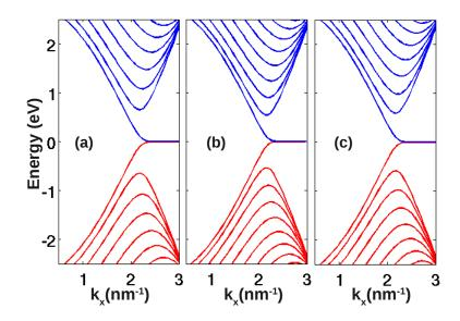
Figure 2.6: Electronic structure of zigzag graphene nanoribbon is shown in three cases with n = 3p, n = 3p + 1 and n = 3p + 2 (p: an integer number).
