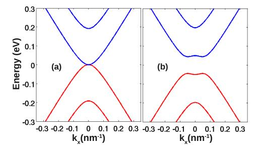
Figure 2.9: Energy bands of bilayer graphene calculated in two cases. Left panel (a):  $\Delta = 0$  and right panel (b):  $\Delta = 50 meV$ .
