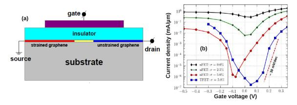
Figure 3.6: Schematic of graphene FET with unstrained/strained junction (a). The channel of the simulated device is based on strained graphene heterostructures. The yellow zone in the graphene layer indicates the transition region between strained and unstrained sections. (b) I- $V_{gs}$  characteristics of simulated graphene FETs at the value of drain voltage  $V_{ds} = 0.1$  V with different strain amplitudes.
