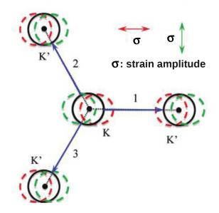
Figure 2.22: Three Raman scattering paths (arrows labeled by 1, 2, 3) from the Dirac cone at K point to the three nearest Dirac cones at K points (circles). The dashed red and green circles indicate the strain-induced movement of the Dirac cone for the zigzag and armchair sample, respectively. The double headed arrows show the strain directions. From M. Huang*et al.* [104]
