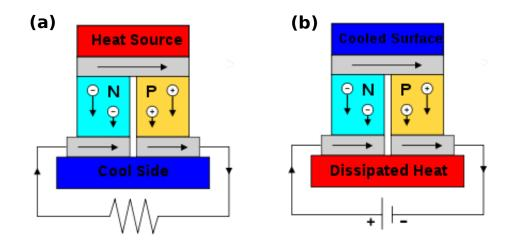
Figure 3.8: Left panel: a thermoelectric circuit composed of materials of different Seebeck coefficient (p-doped and n-doped semiconductors), configured as a thermoelectric generator (a). Right panel: the Seebeck circuit configured as a thermoelectric cooler (b).
