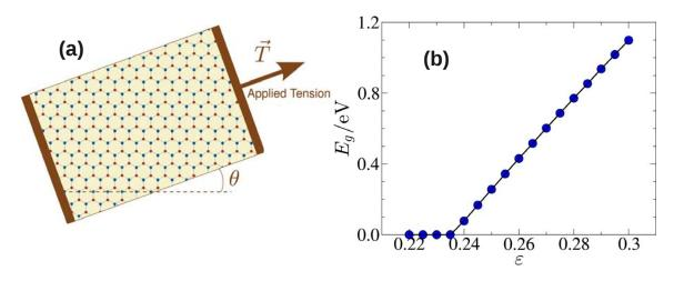
Figure 2.19: Strain is applied on a 2D graphene sheet in (a). The strain dependence of bandgap  $(E_g)$  is shown in (b). From V. M. Pereira *et al.* [71]
