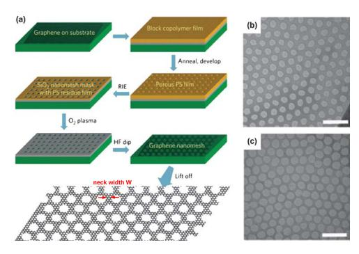
Figure 2.10: Example of fabrication of graphene nanomesh. (a) Schematics of the fabrication process by copolymer lithography. (b), (c) TEM images of graphene nanomesh with average neck width of 11.2 nm and 7.1 nm, respectively. From J. Bai et al. [67]
