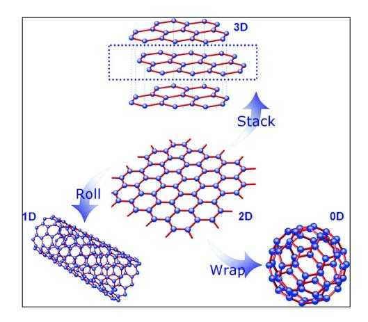
Figure 1.1: Graphene: mother of all graphitic forms. It is a 2D building element for carbon material of all other dimensionalities, i.e., it can be stacked into 3D graphite, rolled into 1D nanotubes or wrapped up into 0D buckyballs (fullerenes  $C_{60}$ ). From X. Wan *et al.* [4]
