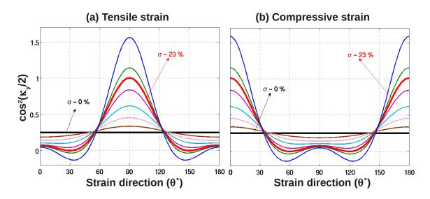
Figure 2.18: Sketch of the relationship (2.29) as a function of strain direction for different strain amplitudes. A strain  $\sigma > 23\%$  is required to open a bandgap in graphene.
