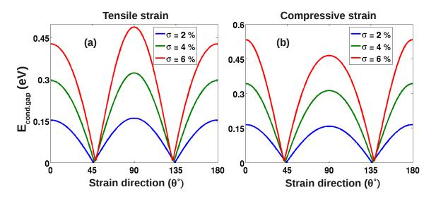
Figure 2.27: Maps of conduction gap in unstrained/strained graphene junctions: tensile (a) and compressive cases (b). The transport is along the armchair directions,  $\phi = 0$ . The strain of 2%, 4%, 6% is considered.
