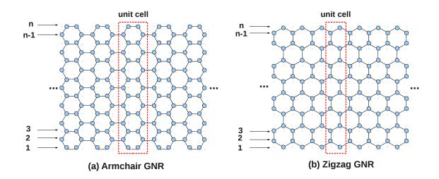
Figure 2.4: Sketch of graphene nanoribbons with (a) armchair and (b) zigzag edges. The GNRs are infinite following the direction of dots and the blocks in red rectangulars are the unit cells. n is number of carbon atom lines along the GNR width.
