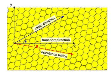
Figure 2.16: Schematic of strained graphene lattice.  $(\theta, \phi)$  are the angles of strain direction with respect to transport direction and of transport direction with respect to armchair direction.
