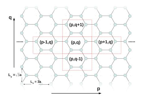
Figure 2.2: Sketch of 2D honeycomb lattice. The central block corresponds to an unit or elementary cell (p,q) consisting of four carbon atoms. The lengths  $L_x = 3a$  and  $L_y = \sqrt{3}a$  are the translation period in p and q directions, respectively. a is the nearest C - C distance.
