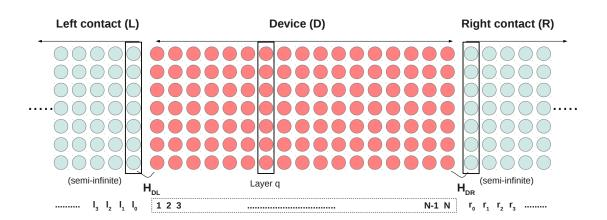
Figure B.1: Schematic of device connected to two semi-infinite contacts. The device and the contacts are split into different layers. Here, one layer only interacts with its nearest neighbor layers.
