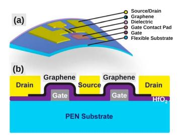
Figure 1.5: Schematic (a) for GFET fabricated on a flexible poly-ethylene naphthalate (PEN) substrate and (b) for cross-sectional schematic of flexible GFET device [39].
