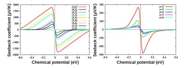
Figure 3.11: Seebeck coefficients of (a) the ZGNR/BNNR superlattices and (b) freestanding ZGNRs at 300 K as a function of the chemical potential felt by electrons. From Y. Yokomizo *et al* [121].
