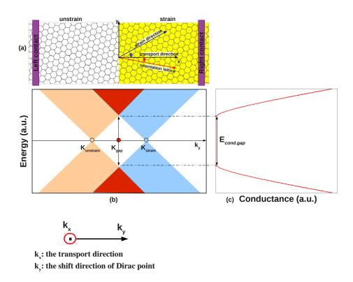
Figure 3.7: (a) unstrained/strained graphene junctions. (b) bandedges illustrating the strain-induced shift of Dirac points along the  $k_y$ -direction that leads to the opening of a conduction gap (c) [chapter 2].
