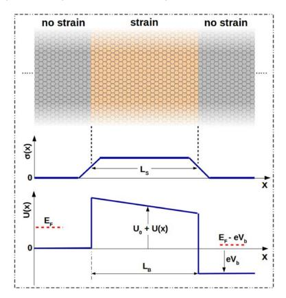
Figure 3.22: Schematic of single potential barrier structures studied in this work. Strain is applied locally in an area of length  $L_S$  and the potential barrier of length  $L_B$  can be generated and controlled by an external gate voltage. The middle panel shows the strain profile  $\sigma(x)$ . The bottom one is the potential energy along the device channel when a bias voltage  $V_b$  is applied.
