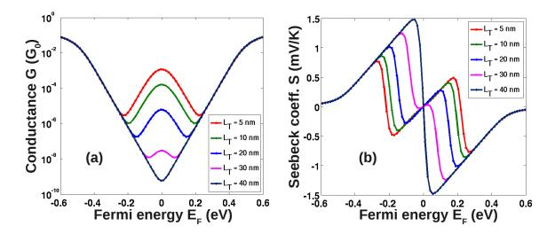
Figure 3.21: (a) conductance and (b) Seebeck coefficient as a function of Fermi energy  $E_F$  for the different lengths  $L_T$ .  $\sigma = 5\%$  and  $\Delta U = 0.5 \, eV$ .
