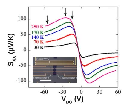
Figure 3.10: Themoelectric power  $(S_{xx})$  as a function of the backgate voltage  $V_{BG}$  in zero magnetic field and at various temperatures: T = 30, 50, 70, 140, 170, and 250K. From Seung-Geol Nam *et al* [132].
