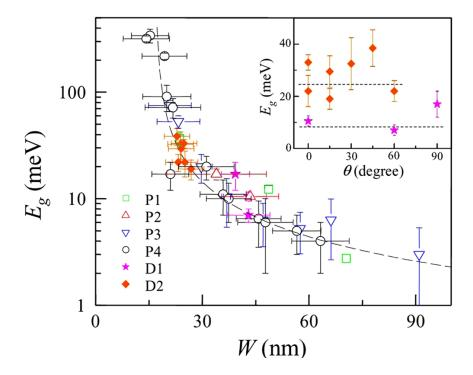
Figure 2.7: Energy bandgap  $E_g$  vs ribbon width W for six device sets with varying orientation. The inset shows  $E_g$  vs relative angle  $\theta$  for the device sets  $D_1$  and  $D_2$ . Dashed line in the inset show the value of  $E_g$  as predicted by the empirical scaling of  $E_g$  vs W. From Y. Han *et al.* [63]
