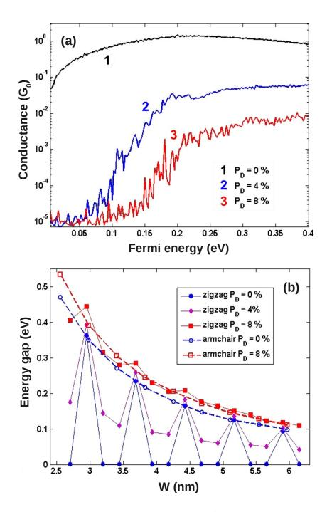
Figure 2.14: (a) Conductance in the unit of  $G_0 = e^2 W_G / hW$  as a function of Fermi energy for different disorder strengths. (b) Energy gap of the GNM lattices as a function of the super-cell lattice constant with disorder effects. From Nguyen *et al.* [98]
