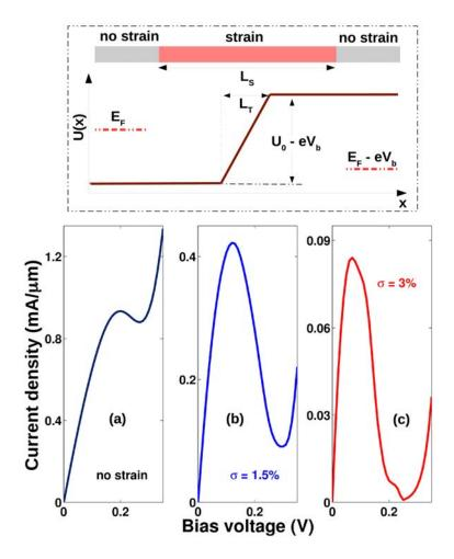
Figure 3.28: The top panel shows the model of graphene p–n junctions studied in this work. The bottom panel shows the I - V characteristics obtained with different strain amplitudes. Other parameters of the device:  $U_0 = 0.5$  eV,  $L_S = 40$  nm and  $L_T = 10$  nm.
