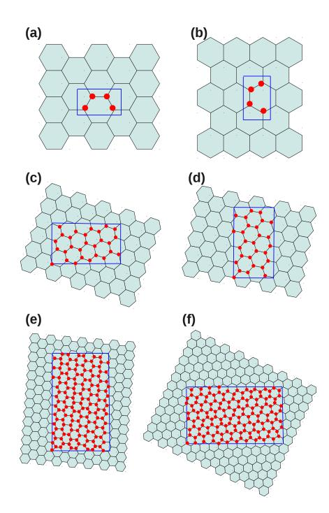
Figure 2.32: Sketch of 2D graphene lattice with different unit cell for six cases of different transport directions from the table. (a)  $\{N_{atom} = 4, \phi = 0\}$ , (b)  $\{N_{atom} = 4, \phi = 30^{\circ}\}$ , (c)  $\{N_{atom} = 28, \phi = 19.1^{\circ}\}$ , (d)  $\{N_{atom} = 28, \phi = 10.9^{\circ}\}$ , (e)  $\{N_{atom} = 148, \phi = 4.7^{\circ}\}$ , and (f)  $\{N_{atom} = 148, \phi = 25.3^{\circ}\}$ .
