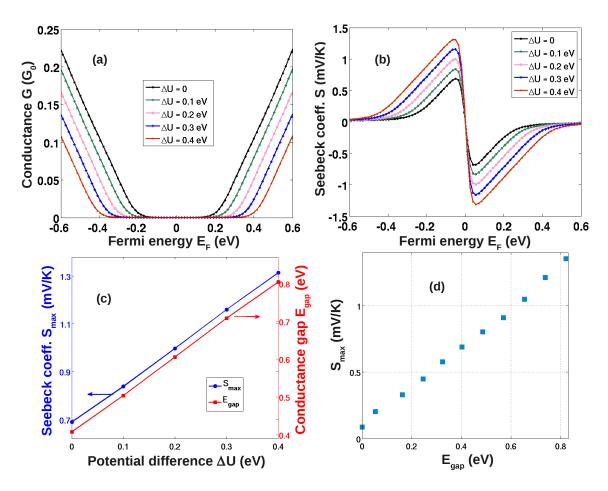
Figure 3.16: (a) Conductance and (b) Seebeck coefficient as a function of Fermi energy  $E_F$  for different  $\Delta U$ . (c) Maximum Seebeck coefficient (Smax) and conduction gap  $(E_{gap})$  as a function of  $\Delta U$ . (d) Smax as a function of  $E_{gap}$ .  $\sigma = 5\%$  is considered here.
