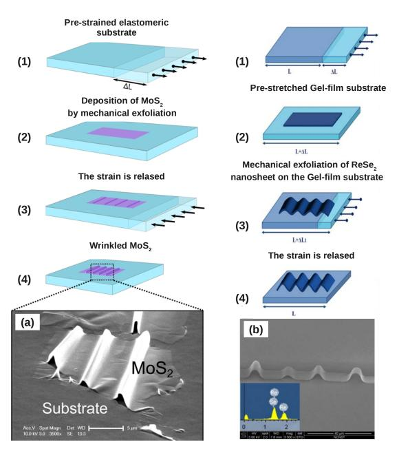
Figure 1.6: Localized uniaxial strain in  $MoS_2$  [26] and  $ReSe_2$  [27].
