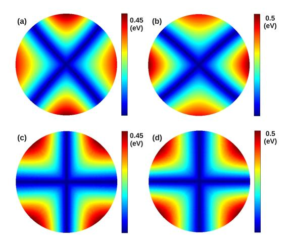
Figure 2.30: Maps of conduction gap in unstrained/strained graphene junctions: tensile (a, c) and compressive cases (b, d). The transport is along the armchair  $\phi = 0$  (a, b) and zigzag  $\phi = 30^{\circ}$  directions (c, d). The strain strength ranges from 0 (center) to 6% (edge of maps) in all cases.
