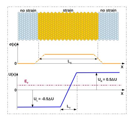
Figure 3.13: Schematic view of the graphene structure investigated in this work, consisting of a PN diode with a locally strained area of length  $L_S$  that covers symmetrically both doped sides. The bottom shows its strain and potential profiles where the doping is characterized by the potential difference  $\Delta U = U_R - U_L$  and the length  $L_T$  of transition region.
