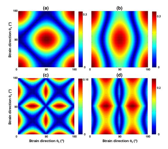
Figure 2.34: Maps of conduction gap obtained in tensile/compressive strained junctions. The transport along the armchair/zigzag directions is considered in (a, b)/(c, d), respectively. The strains  $\sigma_c = 2\%$  and  $\sigma_t = 2\%$  are applied in (a, c) while  $\sigma_c = 1\%$  and  $\sigma_t = 3\%$  in (b, d).
