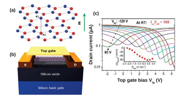
Figure 3.4: Structure of the bilayer graphene FET. Figure (a) shows the bilayer graphene structure in a perpendicular E-filed. A three-dimensional schematic view of the dual-gate bilayer graphene FET in (b). The room temperature transfer characteristics of a dual-gate bilayer graphene FET in (c) [114].
