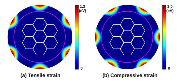
Figure 2.20: Dependence of graphene bandgap on the applied strain and its direction: tensile (a) and compressive (b). The radius from the central point indicates strain strength ranging from 0 (center) to 30% (edge of maps), while the graphene lattice is superimposed to show visibly the strain direction. The pink circle corresponds to the strains of = 23%.
