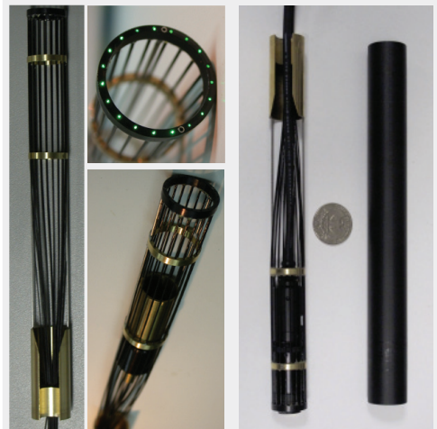
Figure 3. A miniaturized 2D-fluorescent reflectance imaging system especially adapted for oral surgery.
