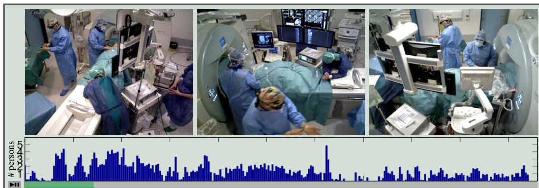
Figure 7.3: Video player tool. The tool shows a bar graph to indicate the number of persons per minute. The bar graph is aligned with the video progress bar, such that the advancement of the progress bar denotes the average number of persons at the corresponding time step.
