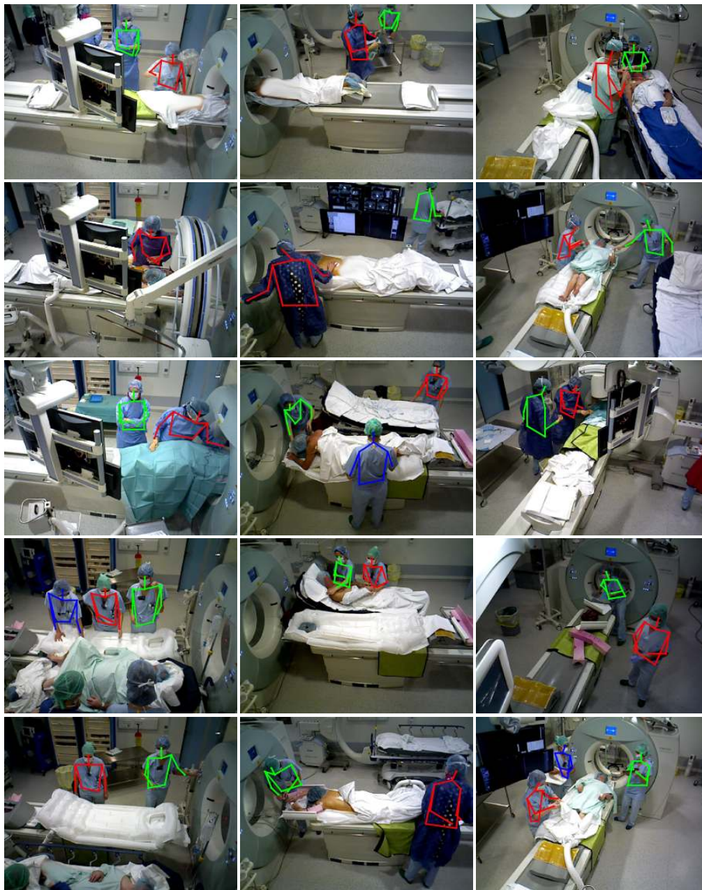
Figure 5.5: Examples of pose estimation results obtained with the proposed 3D pictorial structures approach using \psi_{3D}^4 with I-HOG+HDD. (Picture best seen in color)
