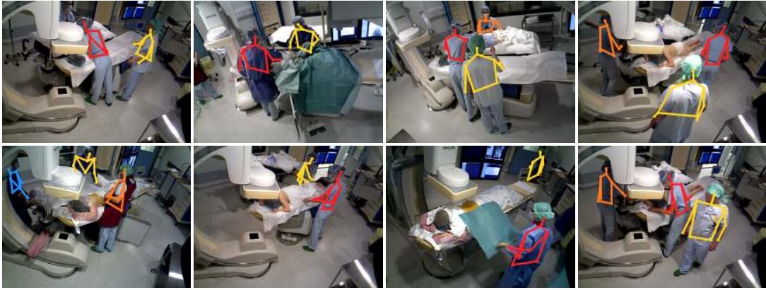
Figure 5.7: Examples of pose estimation results of a model trained on the SV-RGBD-CT dataset and tested on the MV-RGBD-CArm dataset.
