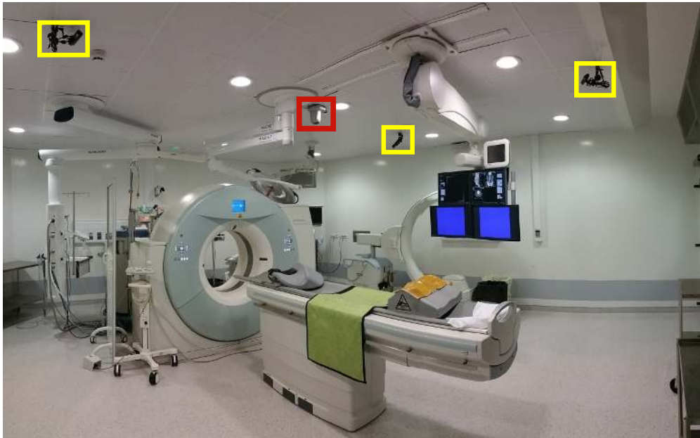
Figure 1.4: A panoramic view of an operating room at NHC Strasbourg, Interventional Radiology Department . Camera positions are highlighted in yellow and red. Yellow boxes indicate the positions of the RGB-D cameras that we have installed in the room to capture the working environment from three viewpoints. The other camera is an RGB camera that has been installed in the room for archiving. It focuses on the bed close to the CT scanner device.
