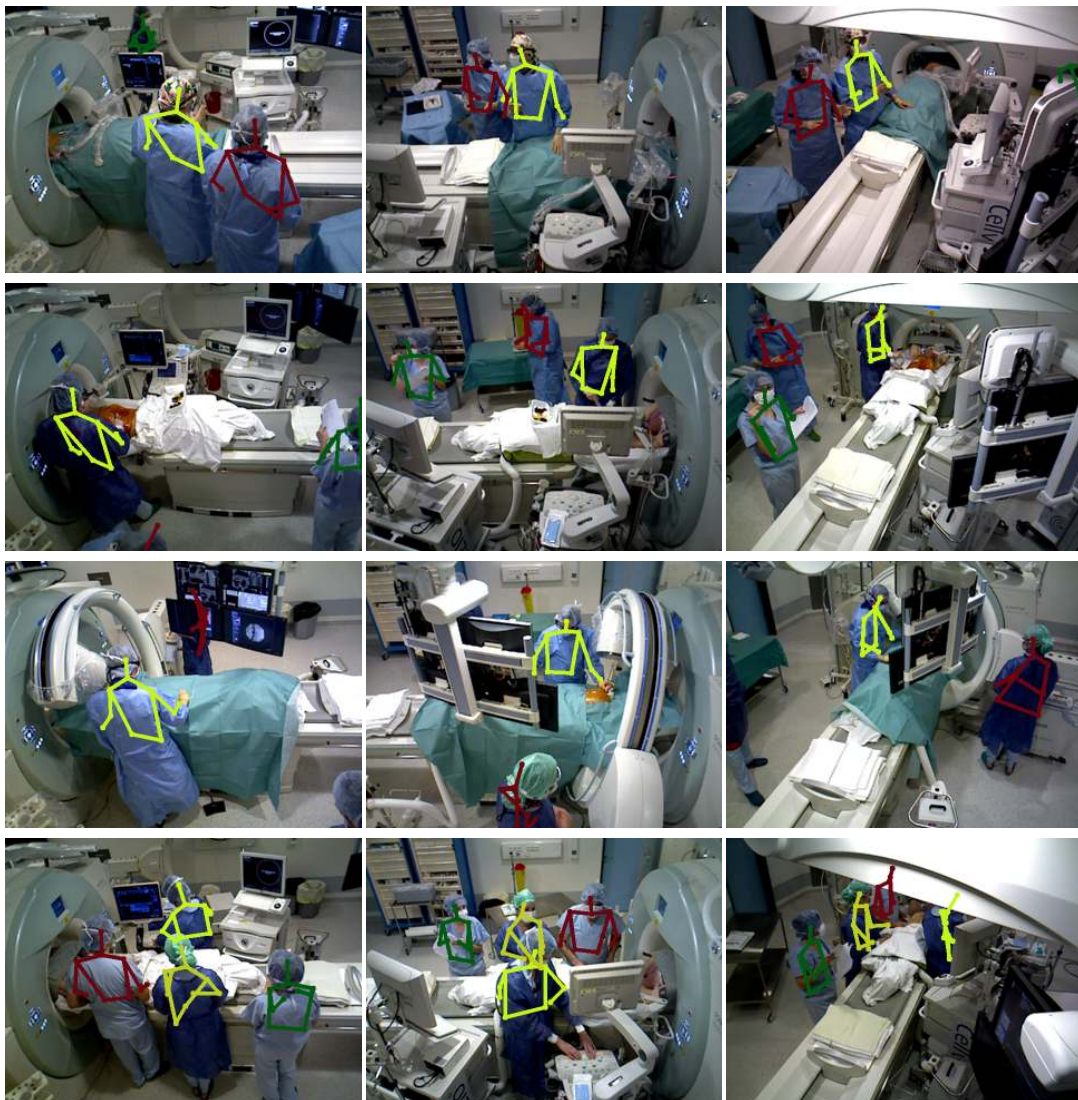
Figure 6.5: Examples of multi-view pose estimation results. Each row shows a multi-view frame. The 3D skeletons obtained after multi-view energy optimization are projected to the views.
