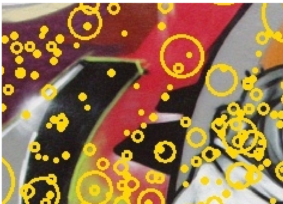
Figure 39: A closer look to SIFT keypoints. This is a part from the upper left side of figure 37. The keypoints detected on the Gaussian pyramid of SIFT can capture either important or very small intensity perturbations. Therefore, keypoints can be found either closer or on edges, corners and blobs but also on areas that for humans look rather homogeneous. The keypoints are represented as yellow circles with their diameter relevant to the scale where they are detected.
