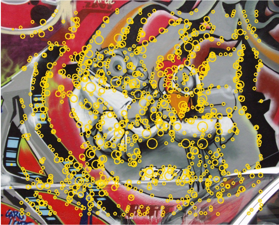
Figure 36: LP-RDFT keypoints. The keypoints are represented as yellow circles with their diameter relevant to the scale where they are detected.
