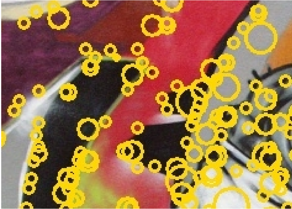
Figure 38: A closer look to LP-RDFT keypoints. This is a part from the upper left side of figure 36. The keypoints detected on the Gaussian pyramid of LP-RDFT capture important intensity perturbations. Therefore, they are more often closer or on edges, corners or blobs. The keypoints are represented as yellow circles with their diameter relevant to the scale where they are detected.
