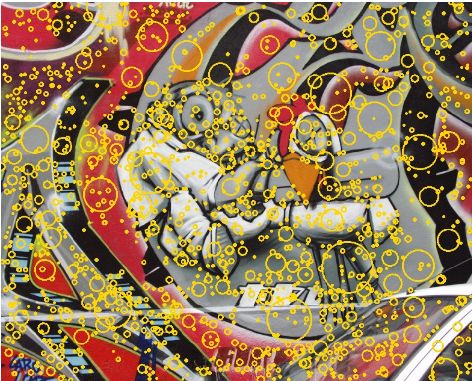
Figure 37: SIFT keypoints. The keypoints are represented as yellow circles with their diameter relevant to the scale where they are detected.
