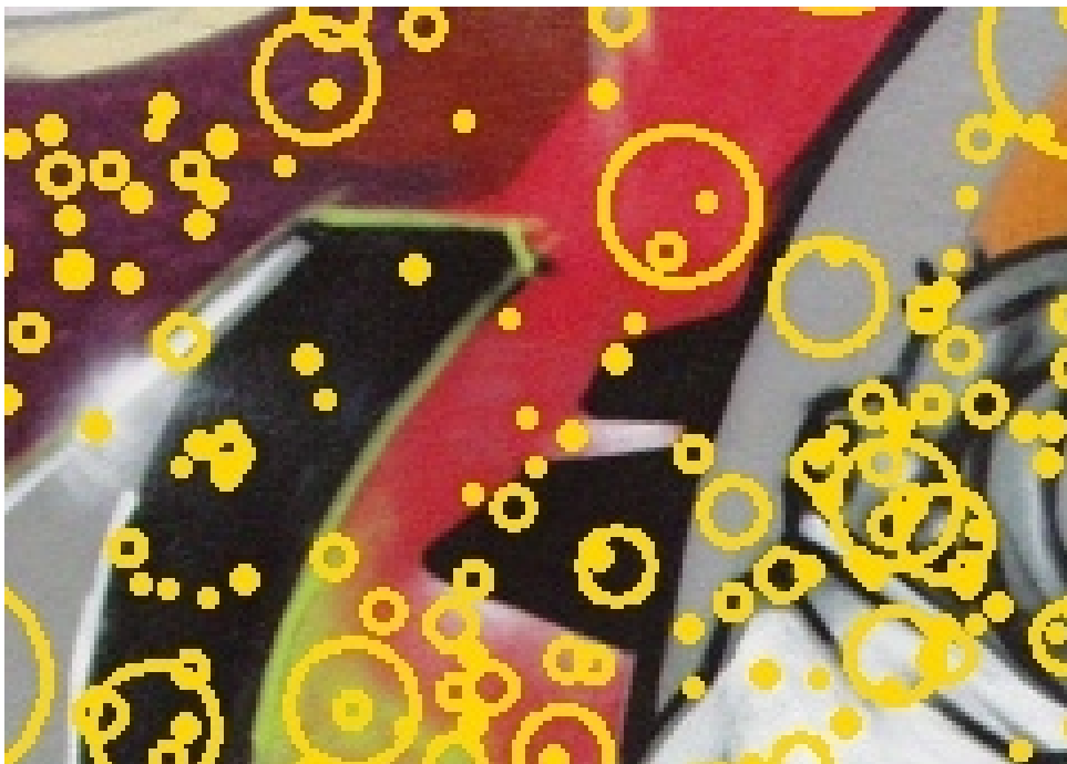
Figure 39: A closer look to SIFT keypoints. This is a part from the upper left side of figure 37. The keypoints detected on the Gaussian pyramid of SIFT can capture either important or very small intensity perturbations. Therefore, keypoints can be found either closer or on edges, corners and blobs but also on areas that for humans look rather homogeneous. The keypoints are represented as yellow circles with their diameter relevant to the scale where they are detected.
