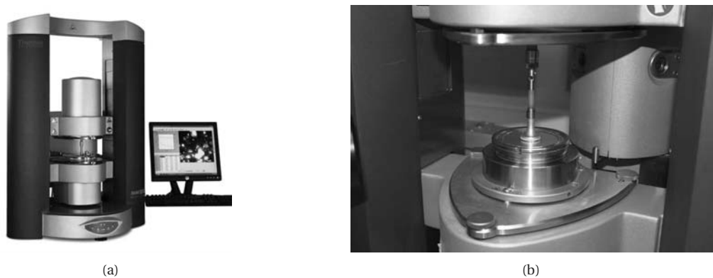
Figure 2.9 – Dynamic shear rheometer HAAKE™ MARS™ from ThermoFisher Scientific: (a) image of the complete device; (b) zoom on the area of interest during an experiment.
