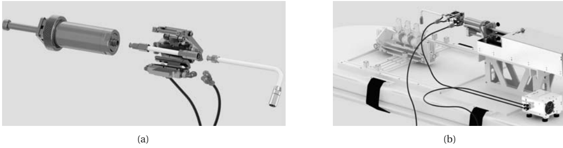
Figure 6.2 – CAD views: (a) clamp used as a water/cement thermal exchanger; (b) experimental scenario with the second prototype.
