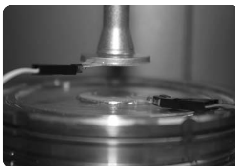
Figure 6.4 – Experimental setup for correlating dielectric and rheological properties of curing bone cement.
