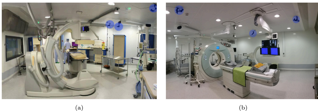
Figure 5.1: Multi-view RGBD camera system in two interventional ORs: (a) C-arm and (b) CT rooms, at the Interventional Radiology Department of University Hospital of Strasbourg. The RGBD cameras mounted on the ceiling are highlighted in blue.
