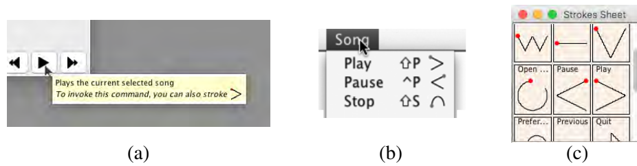
Figure 3.4 : Revealing stroke shortcuts (a) Tooltip , (b) with Menu preview and (c) with a Strokes Sheet
