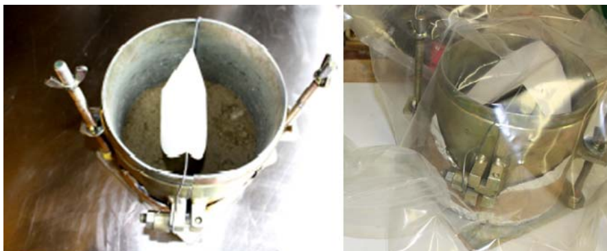
Figure II.12. Cylinder containing the sample of UGM Maraîchères
