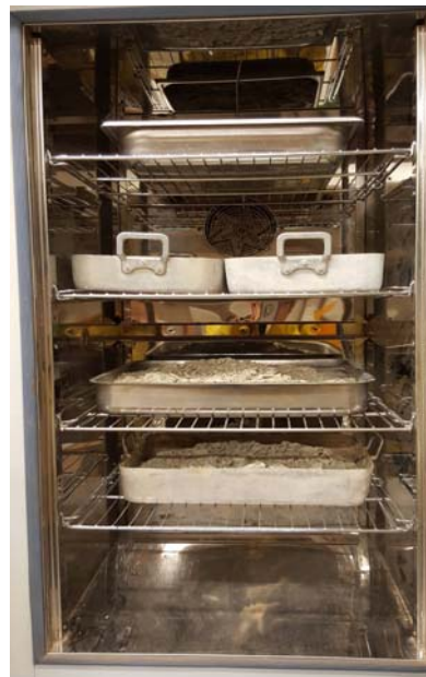
Figure II.16. Soil drying in oven
