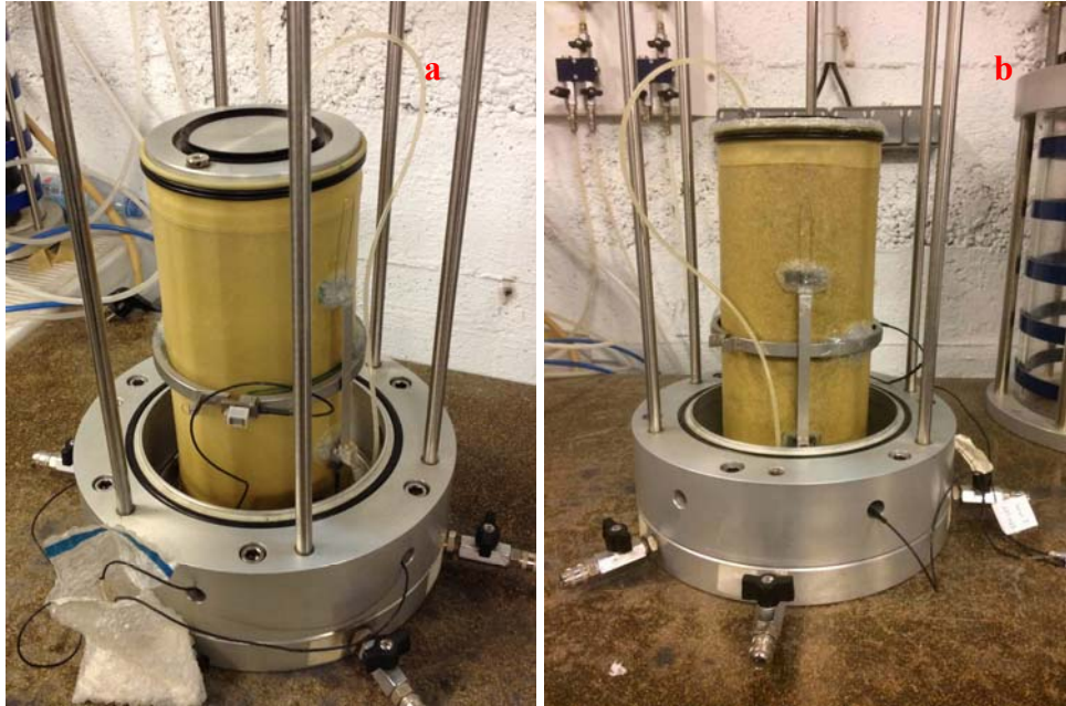
Figure II.21. Samples of RLTT with axial displacement transducers and radial displacement transducer a) Missillac sand b) UGM Maraîchères
